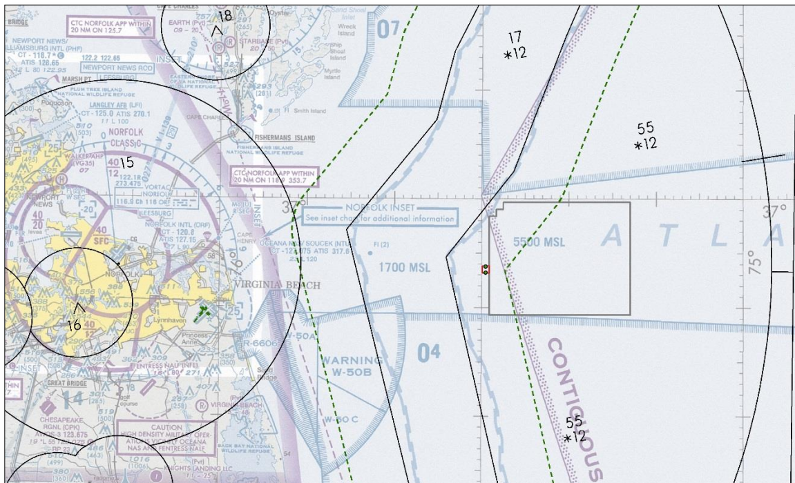
Figure 2: Norfolk (ORF) ASR-9 minimum vectoring altitude chart sectors (black) and 1,200/1,700 foot AMSL sector obstacle evaluation area (hashed green)
