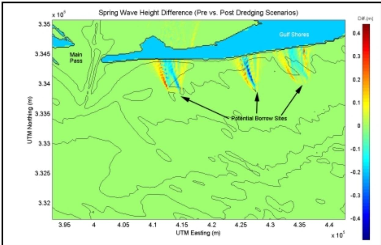
**Figure 5.** Wave height modifications resulting from potential offshore mining at Areas 1, 2, and 3 for a typical spring season. Hot colors (reds) identify areas of increased wave height, while cold colors (blues) identify areas of decreased wave height.
