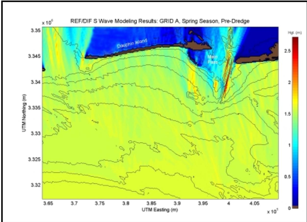
**Figure 2.** Spectral wave modeling results for existing conditions and a typical spring season.
