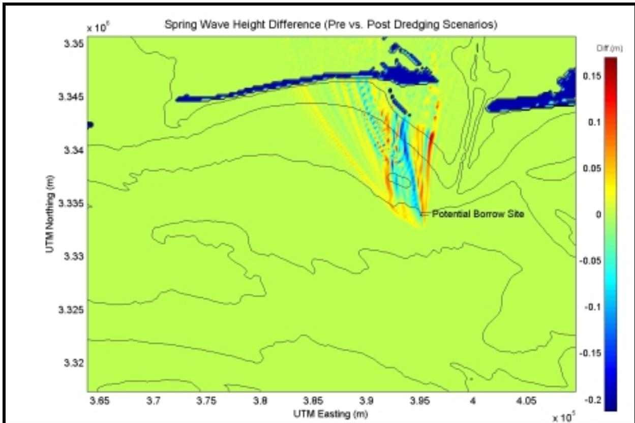
**Figure 4.** Wave height modifications resulting from potential offshore mining at Area 4 for a typical spring season. Hot colors (reds) identify areas of increased wave height, while cold colors (blues) identify areas of decreased wave height.
