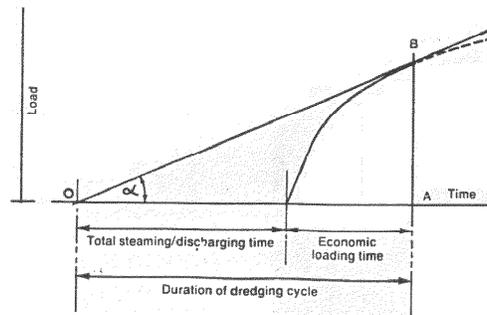
Figure 5. Schematic of Estimating Optimum Overflow Duration for Trailing Suction Hopper Dredge.
