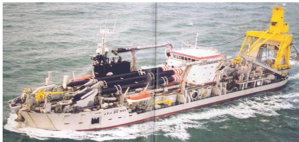
Figure 3. Self Propelled Cutter Suction Dredge JFJ de Nul (Courtesy of Jen de Nul)
