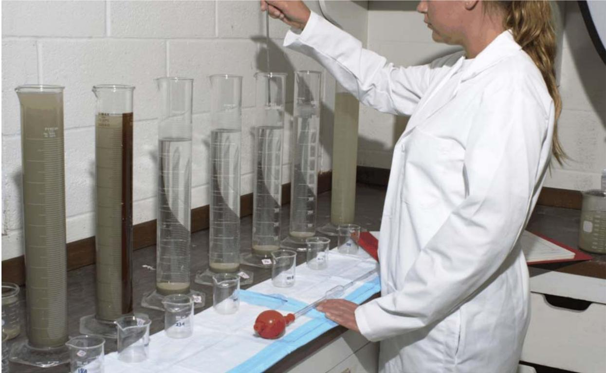
Figure A5 Mixing silt and clay as part of pipette analysis to determine silt and clay contents
