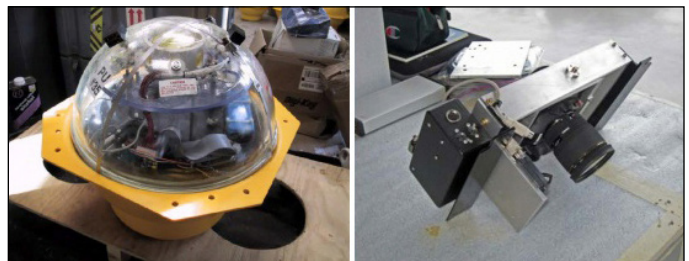
Equipment used for monitoring whales. Left: acoustic recording instrument. Right: camera and mounting equipment.
