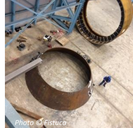
Photo © Fistuca Blue piling hammer manufact. for full scale test
