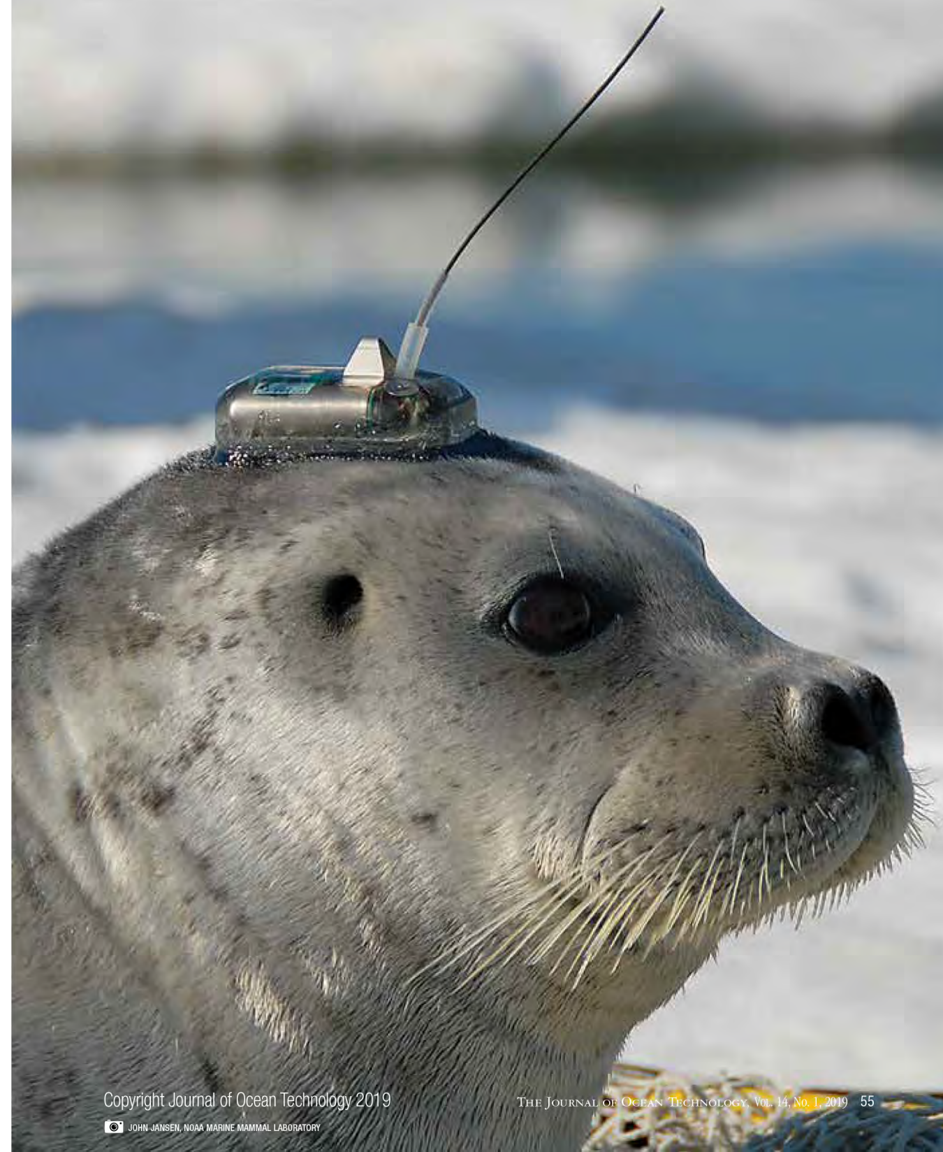
Figure 3: An adult seal, from a BOEM study, with a head-mounted, satellite-linked, geo-locating data recorder in Kotzebue Sound, Alaska.
