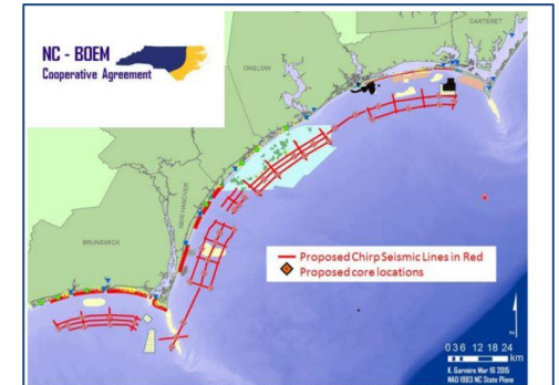
Fig. 4. Map of prioritized seismic and core collection in NC for 2015 CB&I data collection based on existing data availability.
