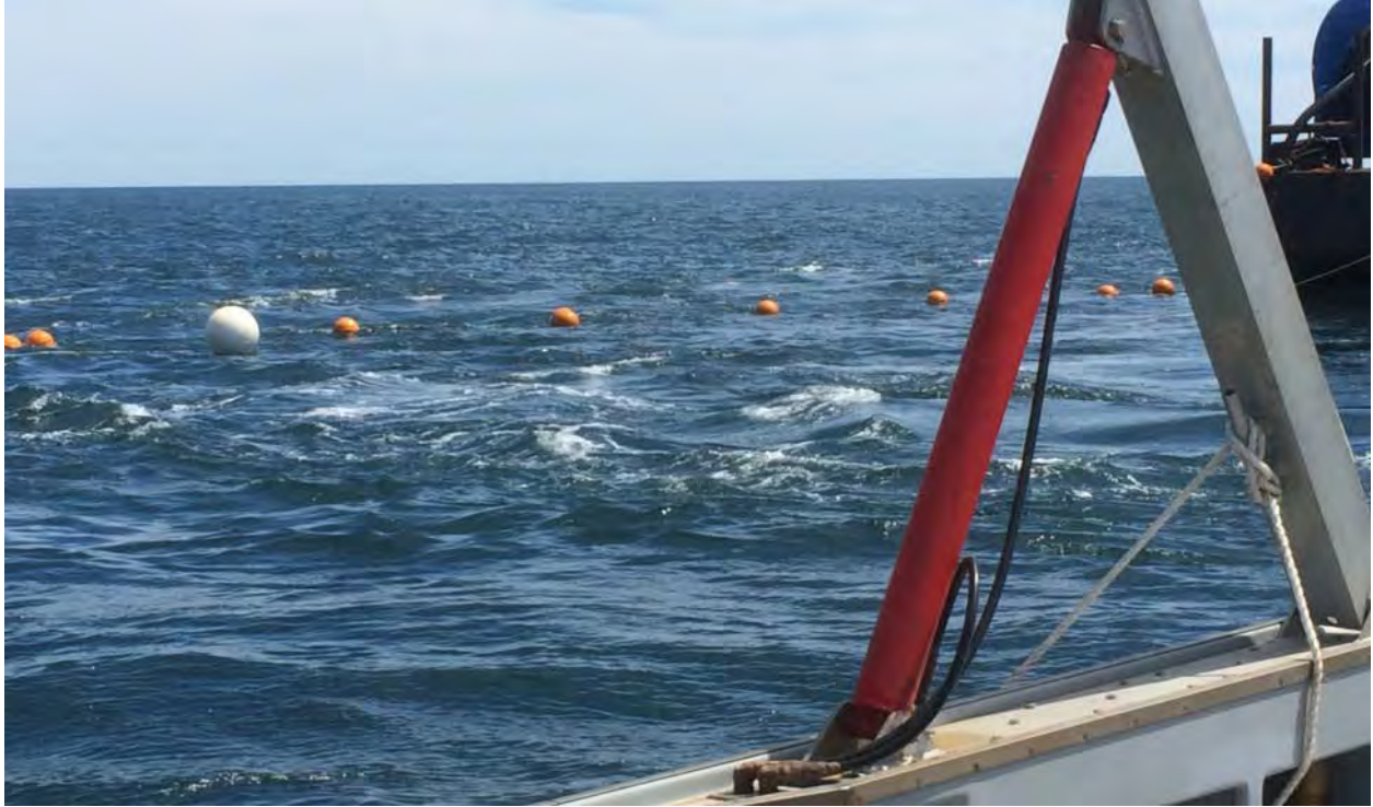
Figure 24. Turbulence around the jet plow caused by vessel thrusters
