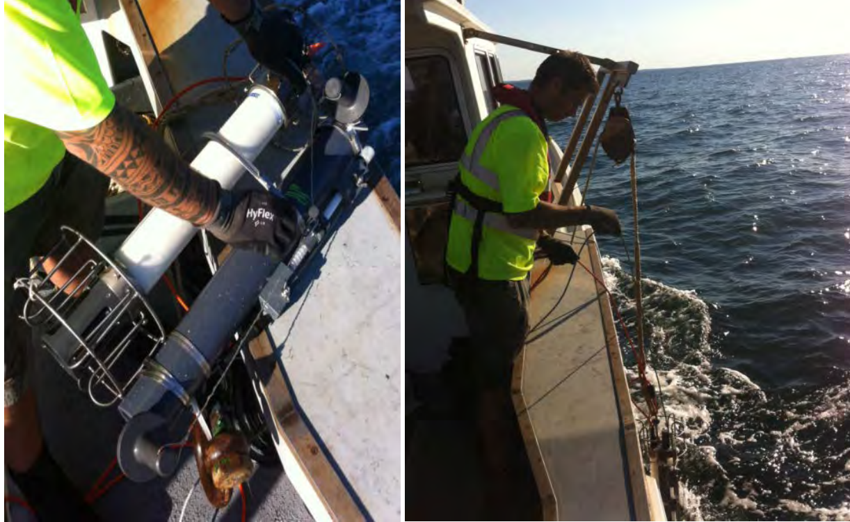
Figure 19. Idronaut profiler and Niskin water sampling bottle being prepared for deployment (left), Idronaut profiling and water sampling activities aboard Jamie Hanna (right)
