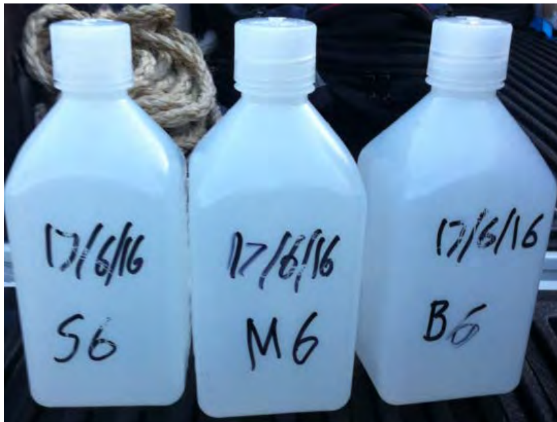
Figure 20. Water samples taken at the surface, middle and bottom of the water column, 120 meter astern of the jet plow showing low sediment concentration
