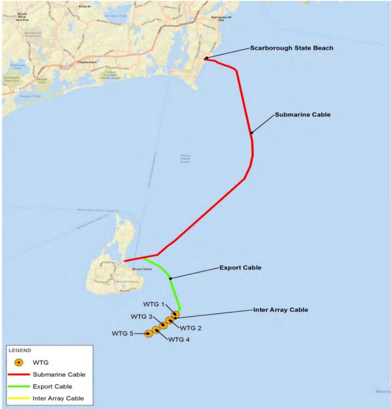
Figure 2. BITS Cable Route
