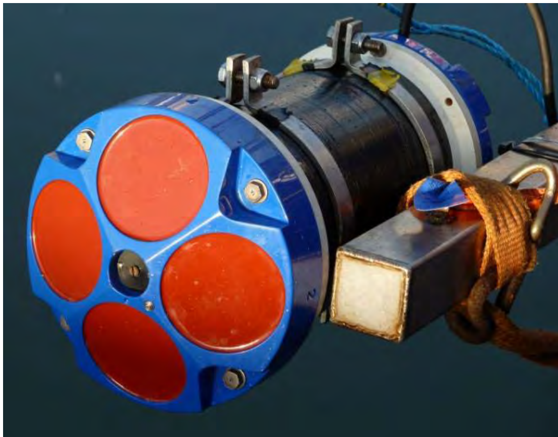
Figure 17. RDI ADCP configured on pivoting arm
