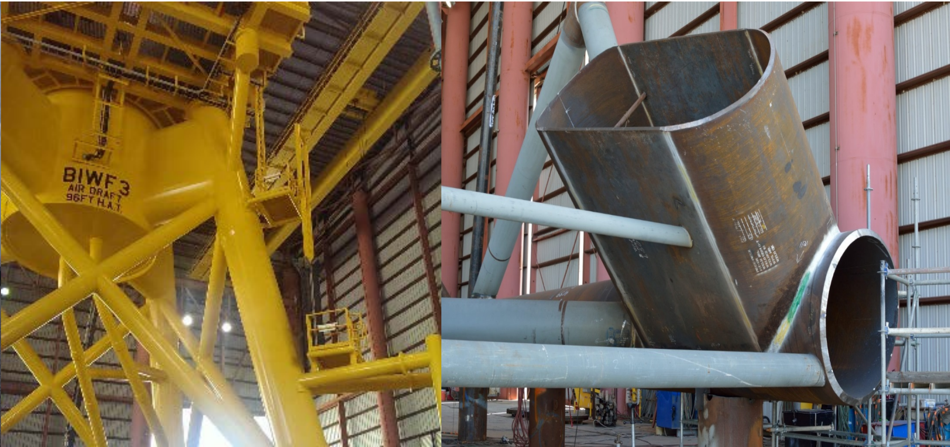
'RACE TRACK' BRACE FRAMING
