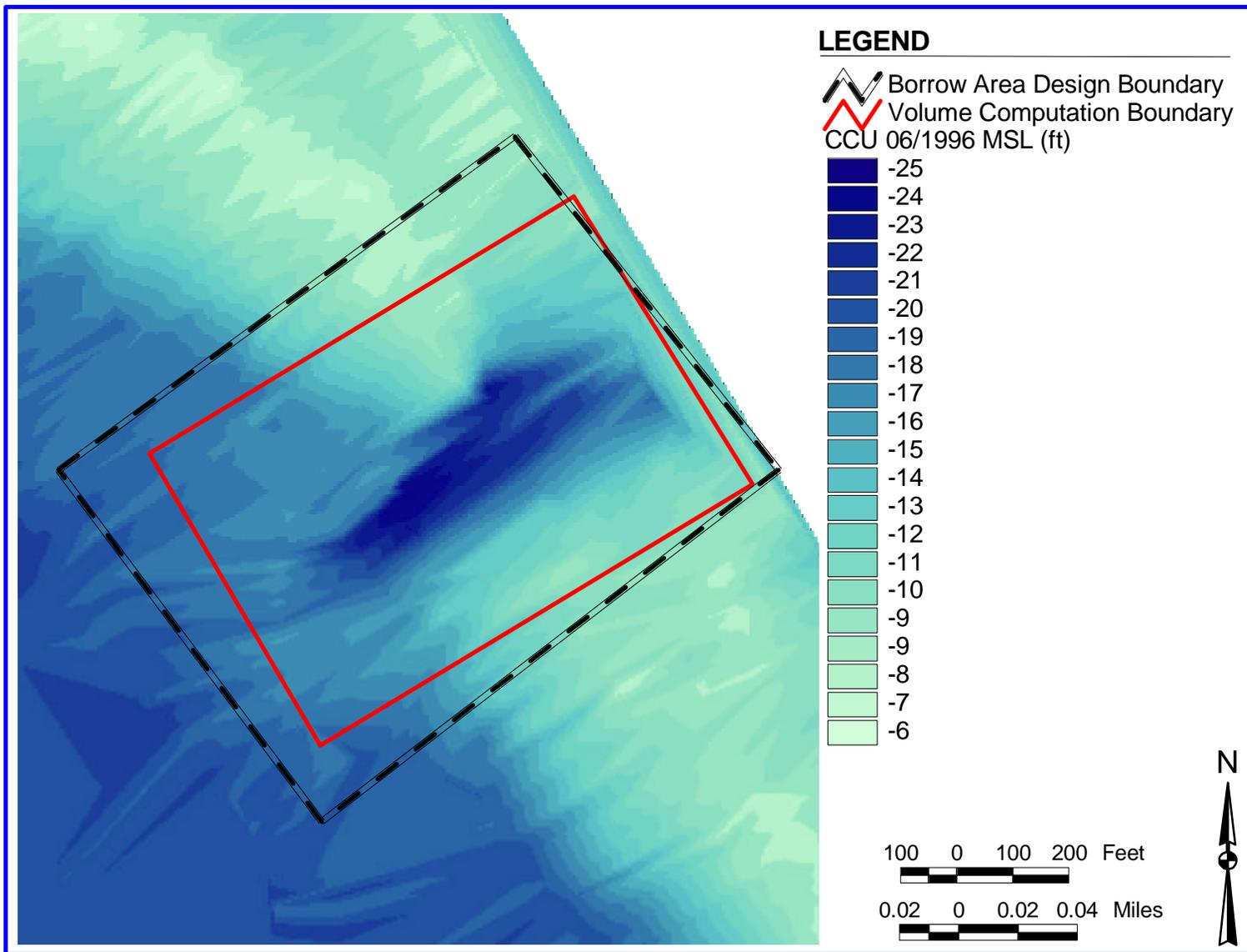
Figure 29. Edisto Island borrow site with bathymetric data from the 1996 post-construction survey conducted by Coastal Carolina University.
