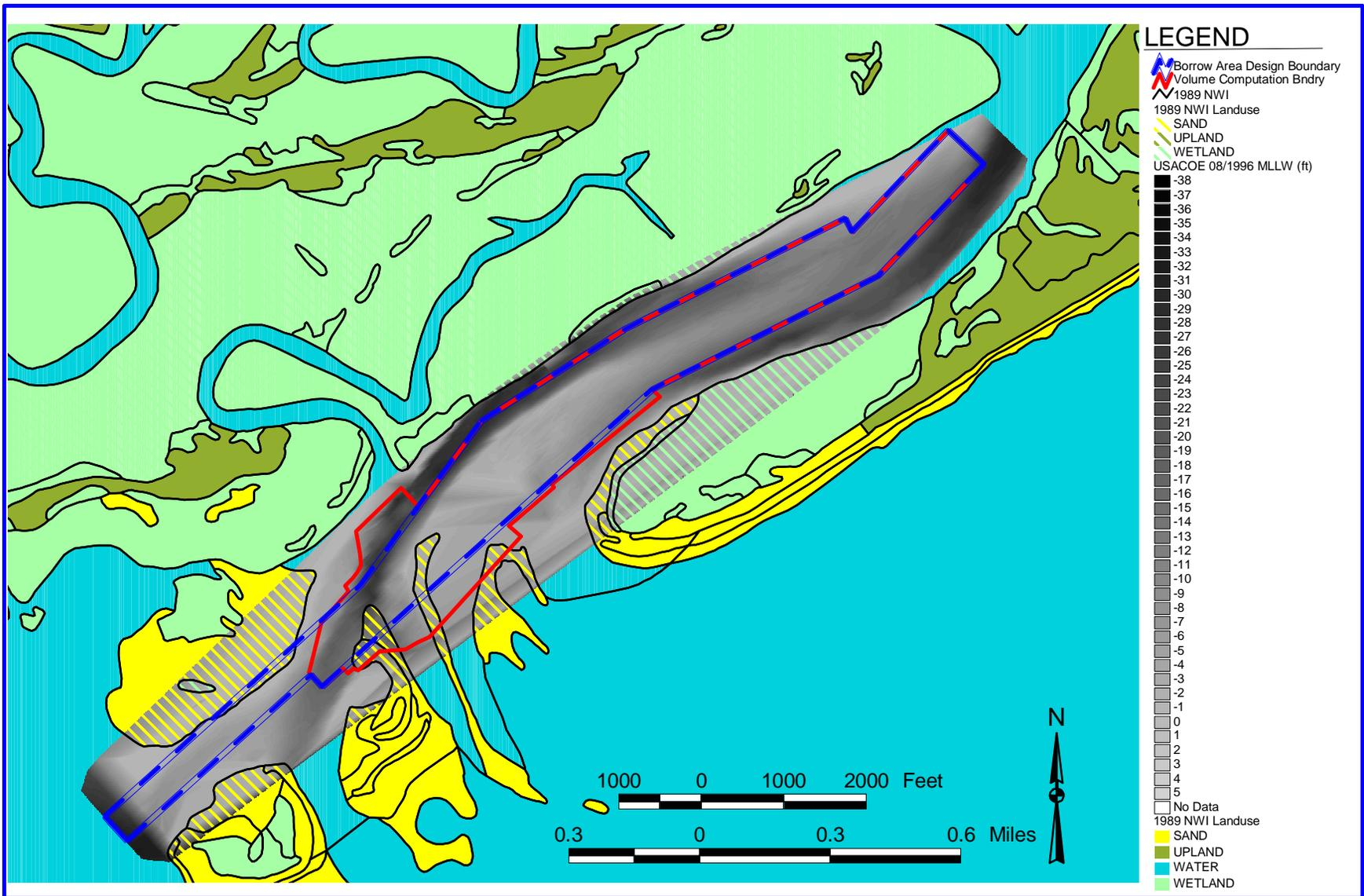
Figure 17. Folly River borrow site with bathymetric data from the USACOE post-construction survey (8/96).
