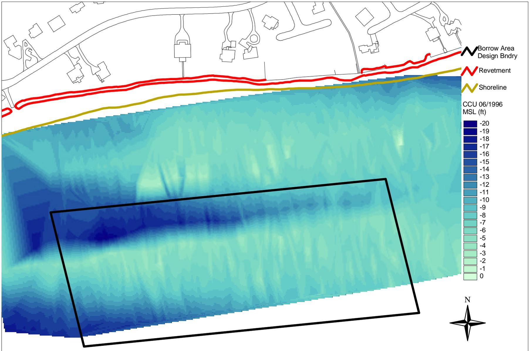
Figure 31. Seabrook Island borrow site with bathymetric data from the 1996 post-construction survey conducted by Coastal Carolina University.
