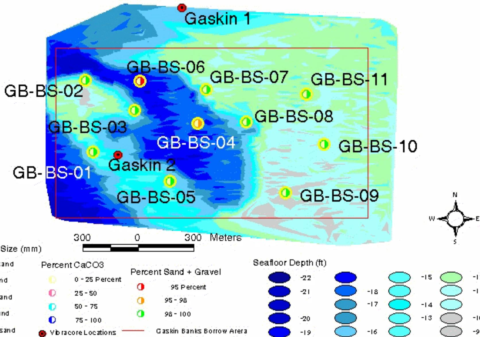
Figure 26. Location of stations samples at the Gaskin Banks borrow site by Coastal Carolina University during the 1996 survey, with summary information on sediment grain size and composition overlaid on the 1996 bathymetry data.
