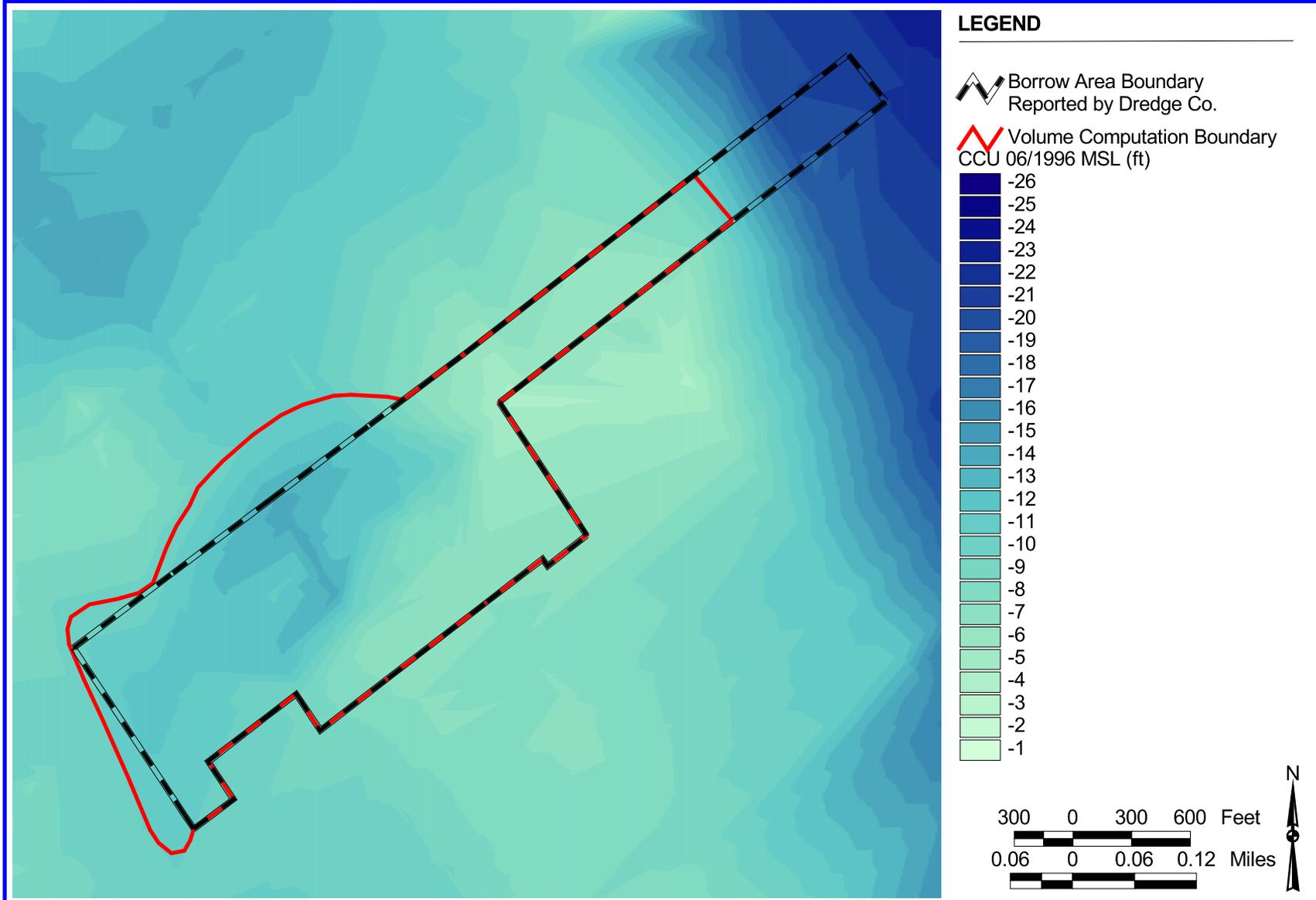
Figure 19. Joiner Bank borrow site with bathymetric data from the 1994 post-construction survey conducted by Coastal Carolina University.
