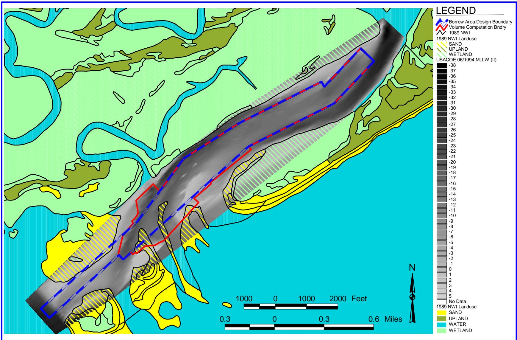
Figure 15. Folly River borrow site with bathymetric data from the USACOE post-construction survey (6/94).
