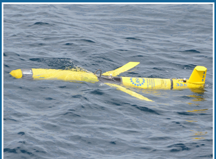
A Slocum glider is an independently mobile platform that can carry various technologies to collect and transmit oceanographic and biological data. Photo: Suzanne Yin, NOAA.
