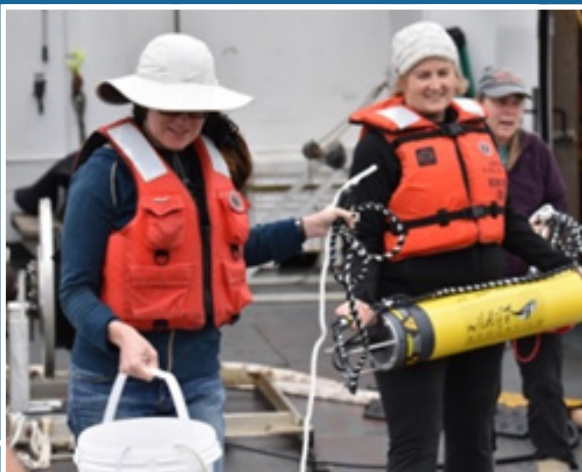
Scientists deploying a Drifting Acoustic Spar Buoy Recorder (DASBR) to listen for deep diving whales. Photo: Greg Sanders, BOEM
