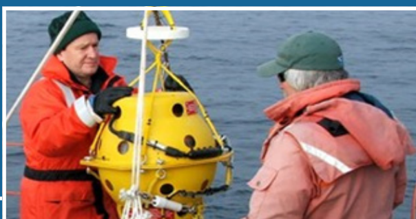
Acoustic buoy (Marine Acoustic Recording Unit [MARU]), Photo taken under ESA Research Permit # 1576. Photo: Heather Haas, NOAA/ NEFSC.
