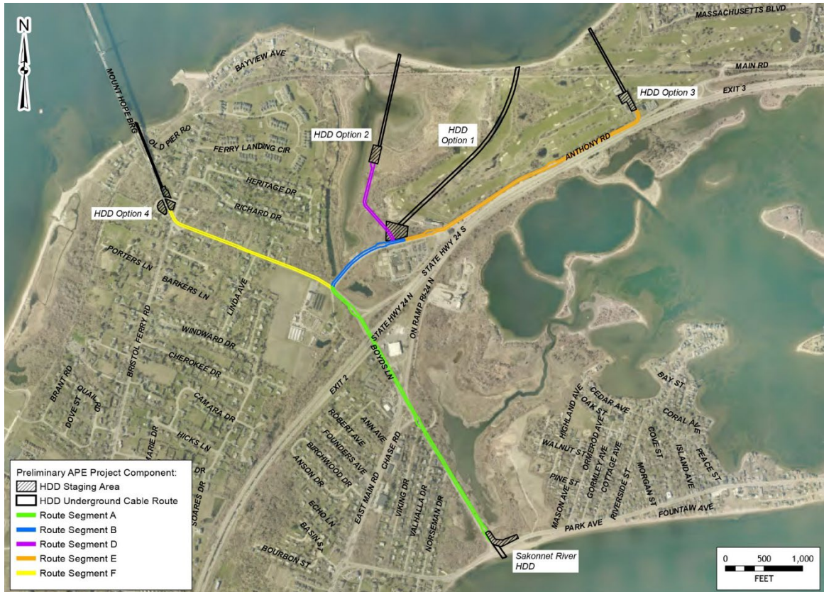
Figure 1. Proposed onshore cable routes and HDD locations for the SouthCoast Wind Aquidneck Island (Portsmouth) Landfall.
