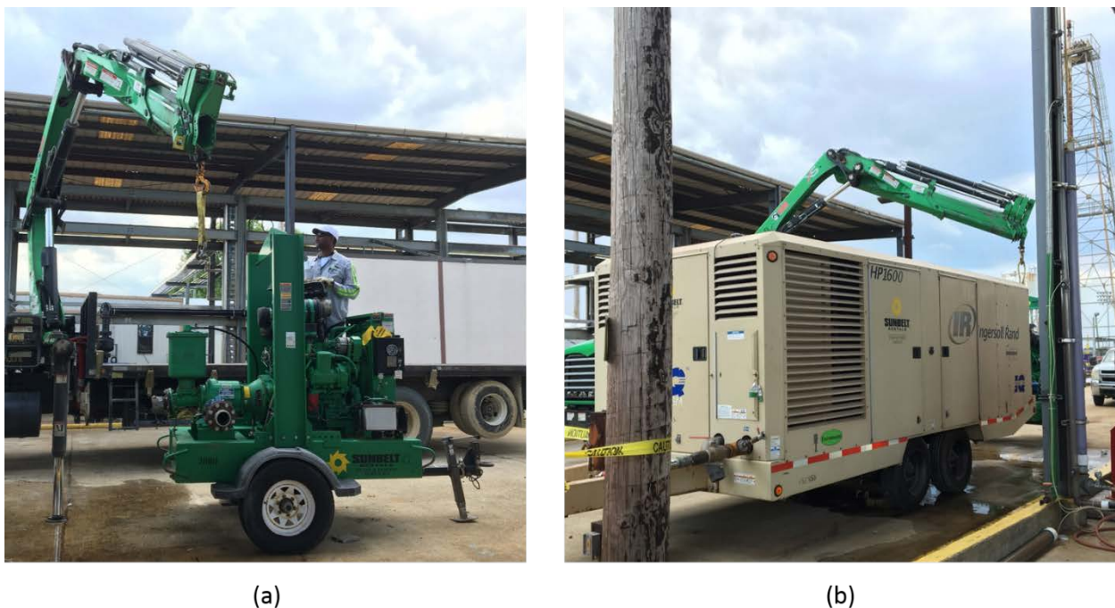
Figure 6: Equipment used to achieve higher flow rates, being them (a) the large pump; and (b) the large compressor.
