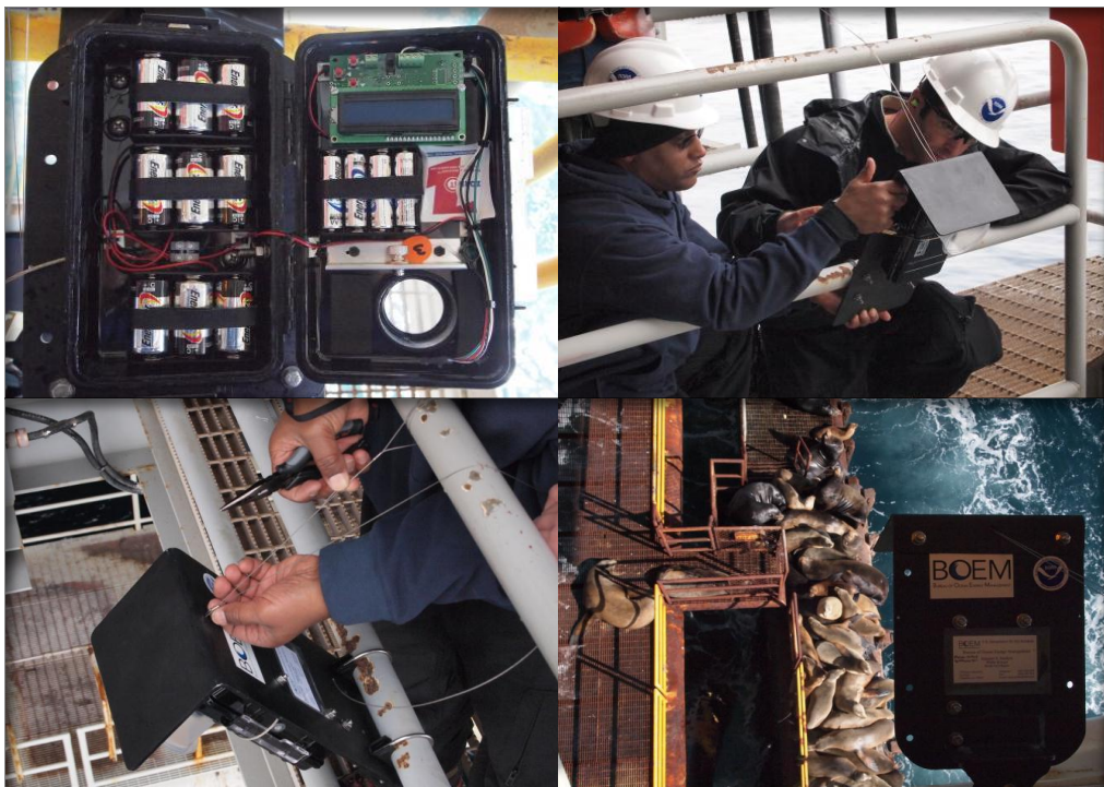
Figure 3. Digital automated time-lapse camera systems (developed by Trail Watcher Game Cameras; Monticello, Georgia) that were installed on five gas and oil platforms offshore southern California and programmed to take images between January 2013 and January 2015. The systems consisted of a timing circuit, a camera, and battery bank. They were placed in locations where most areas where pinnipeds could be viewed were covered.
