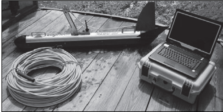
Figure D-21. Example of a Representative Side-Scan Sonar System (EdgeTech, 2011).
