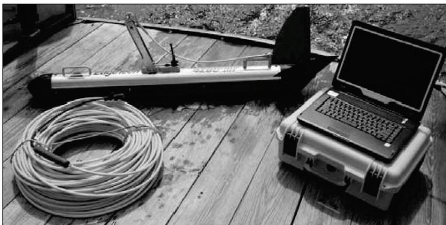
Figure D-21. An Example of a Representative Side-Scan Sonar System. Source: EdgeTech (2011).
