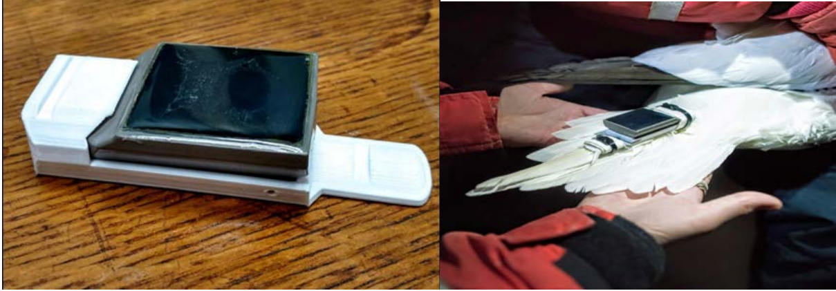
Figure 6-5. Left: Tag adapter created with a 3-D printer, designed to securely attach solar-powered transmitters close to tail feathers close to the body of gannets. Right: finalized package attached to NOGA_12.
