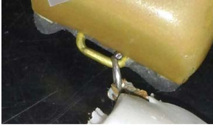
Figure 6-3. Method of attaching silicone harness to transmitter using stainless steel rings that failed within 60 days.
