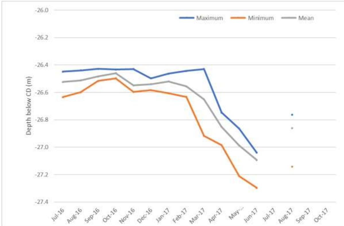
Figure 81. SE Beam 1 scour depth.
