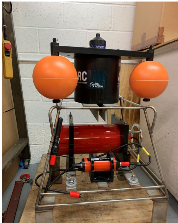
Figure 3. Example of a multi channel hydrophone array measuring 2m x 2m and weighing ~150kg
