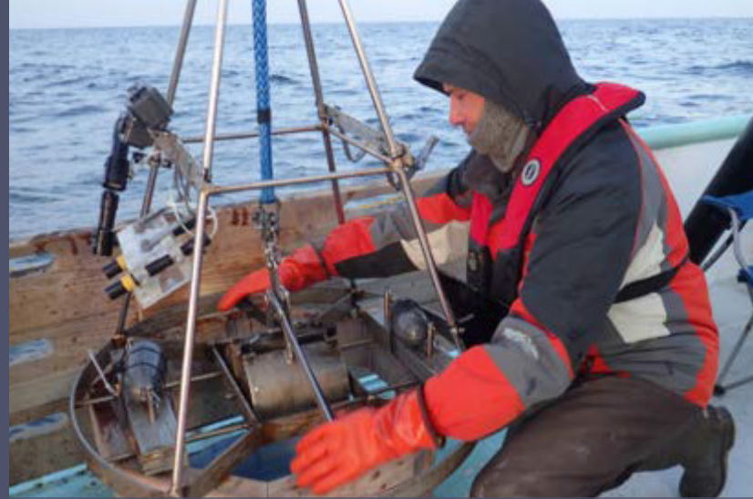
NCCOS scientist opening the mapping and model validation sampler to release the sediment sample into the bin below
