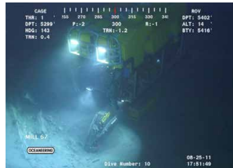
Free swimming ROV with dredge attachment. Oceaneering 12 Inch XL Electric Dredge. Image courtesy of Oceaneering, 2017.
