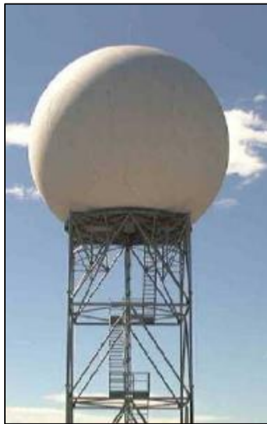
Figure 22 - WSR-88D Weather Surveillance Radar
