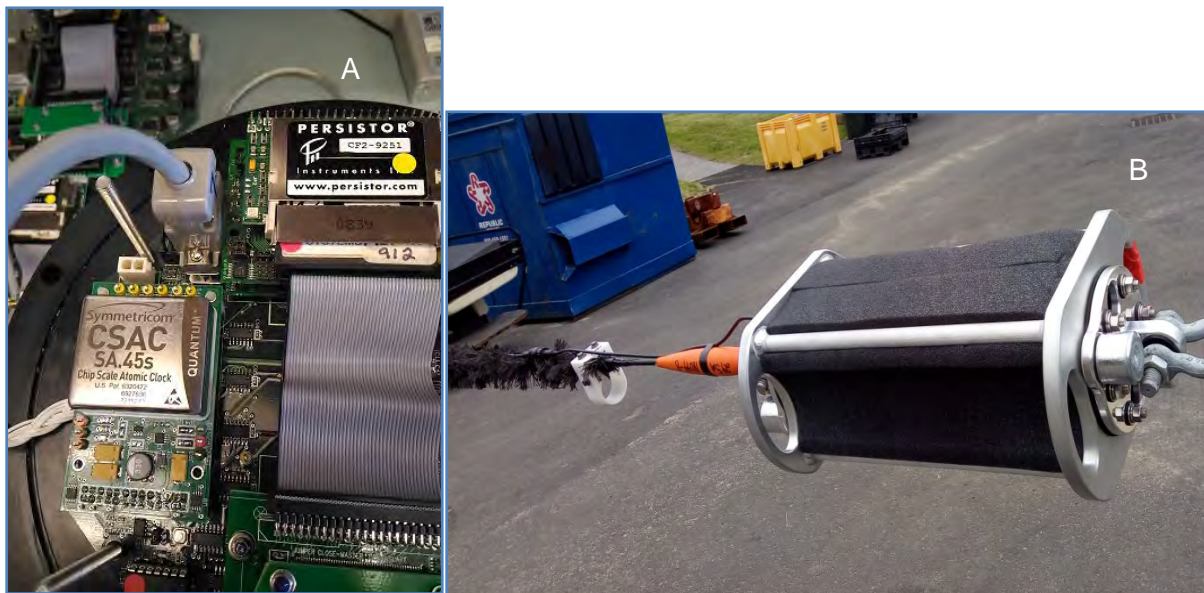
Figure B-5. A) CSAC-SHRU electronic board(A) and (B) Hydrophone cage with flow shield and hairy fairing wire (B)
