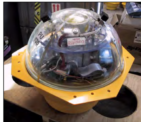
Figure 5. External and internal views of a marine autonomous recording unit (MARU).
