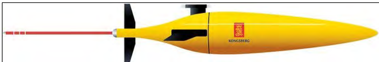
Figure 7. Seaglider™ autonomous underwater vehicle.
