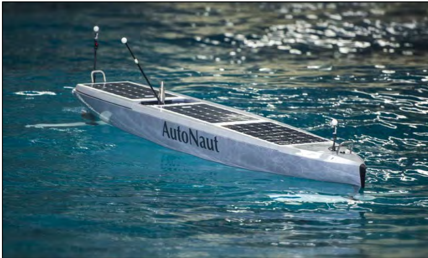
Figure 9. AutoNaut® with towed array–wave propelled autonomous surface vehicle.
