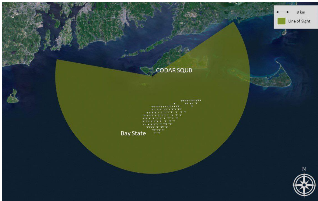
Figure 64 - Line of Sight plot for the SQUB SeaSonde located on Martha’s Vineyard with reference to the Bay State farm.
