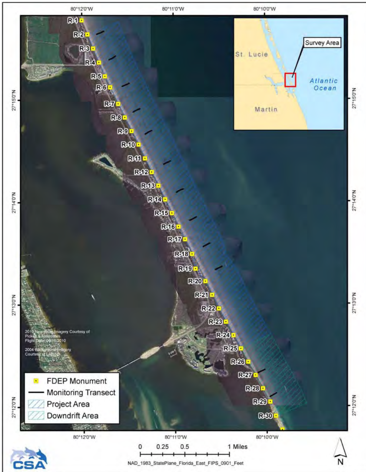
FIGURE 3.4-2 SURVEY AREA OVERVIEW SHOWING PERMANENT CROSS-SHORE TRANSECTS ESTABLISHED AND SURVEYED DURING THE HUTCHINSON ISLAND SHORE PROTECTION PROJECT 2010 HARD BOTTOM BASELINE SURVEY; MARTIN COUNTY HURRICANE AND STORM DAMAGE REDUCTION PROJECT, HUTCHINSON ISLAND, FLORIDA
