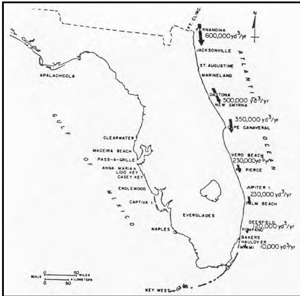
Figure 4. Estimates of net annual longshore sand transport along the east coast of Florida derived primarily from USACE documents (from Dean and O'Brien, 1987; Dean, 1988).
