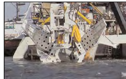
Figure 3 Lowering Plow with Share Open
