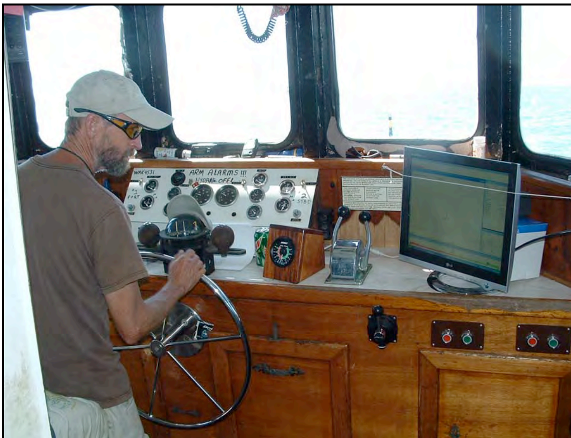
Figure 15. Computer navigation system located at the research vessel helm.
