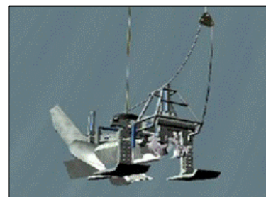
Figure 3 Lowering Plow with Share Open
