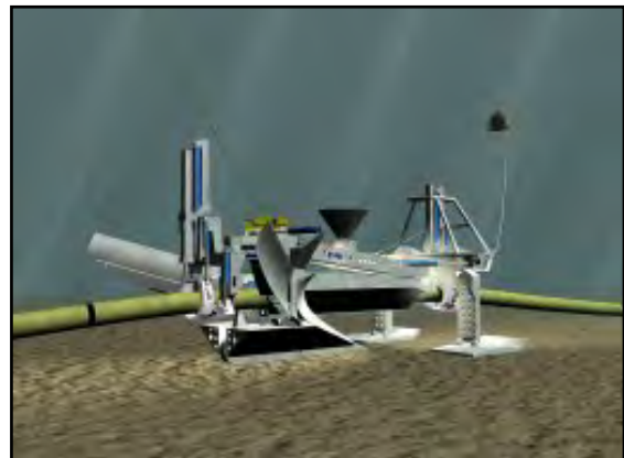
Figure 5 Monitoring and Adjustment of Ditch Being Cut
