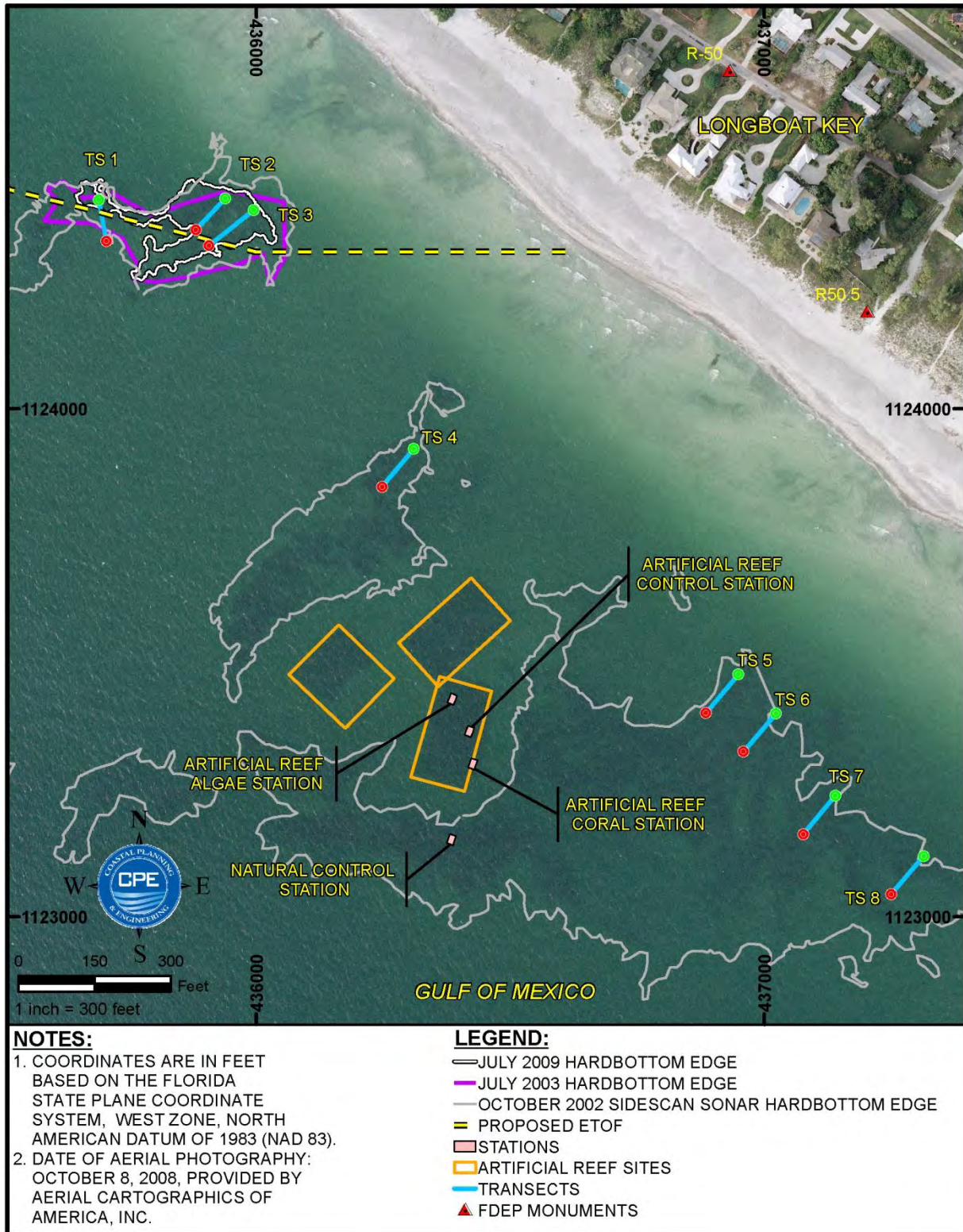
Figure 2. Nearshore natural hardbottom monitoring transects and mitigative artificial reef located between R49.5 and R51.5 on Longboat Key. Hardbottom edge delineations presented from 2002 sidescan sonar and 2003 and 2009 in situ diver verification.
