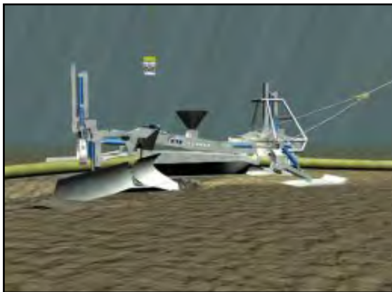
Figure 4 Pipeline Raised into Plowshare
