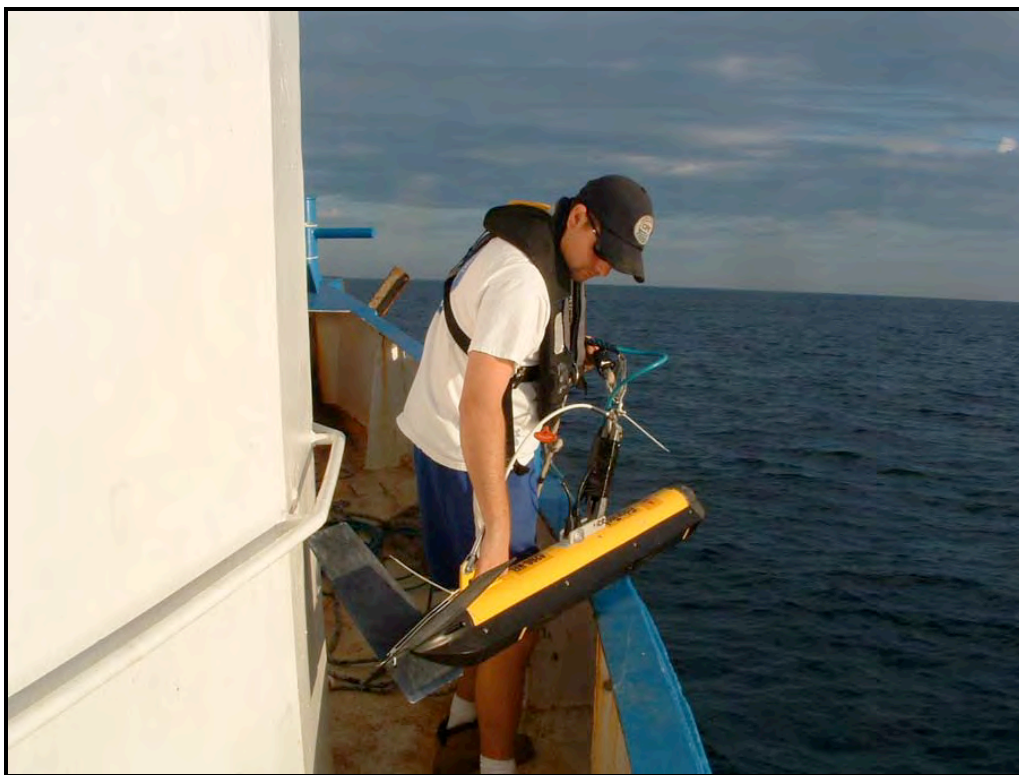
Figure 13. Launching the EdgeTech 4200-HFL sidescan sonar.
