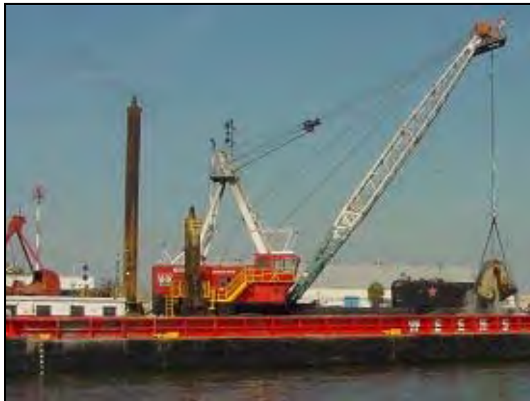
Figure 3-2 Conventional Spudded Leg Clamshell Dredge (courtesy of U.S. Army Corps of Engineers)
