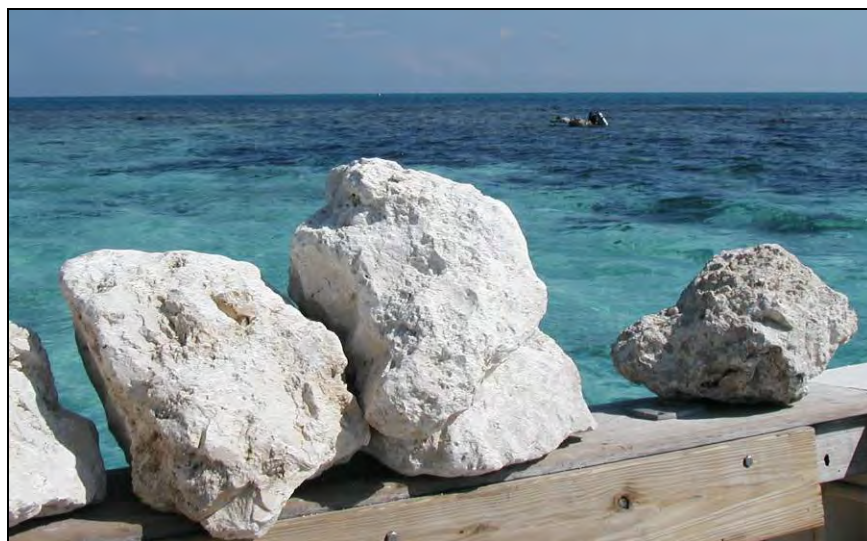
Figure 14 Limestone Boulders (Size Range of 1 to 1.5 feet [0.3 to 0.5 meters]) Representative of Those Suggested for Mitigation to be Used to Mimic the Low-relief Structure of the Natural Hard Bottom Habitat
