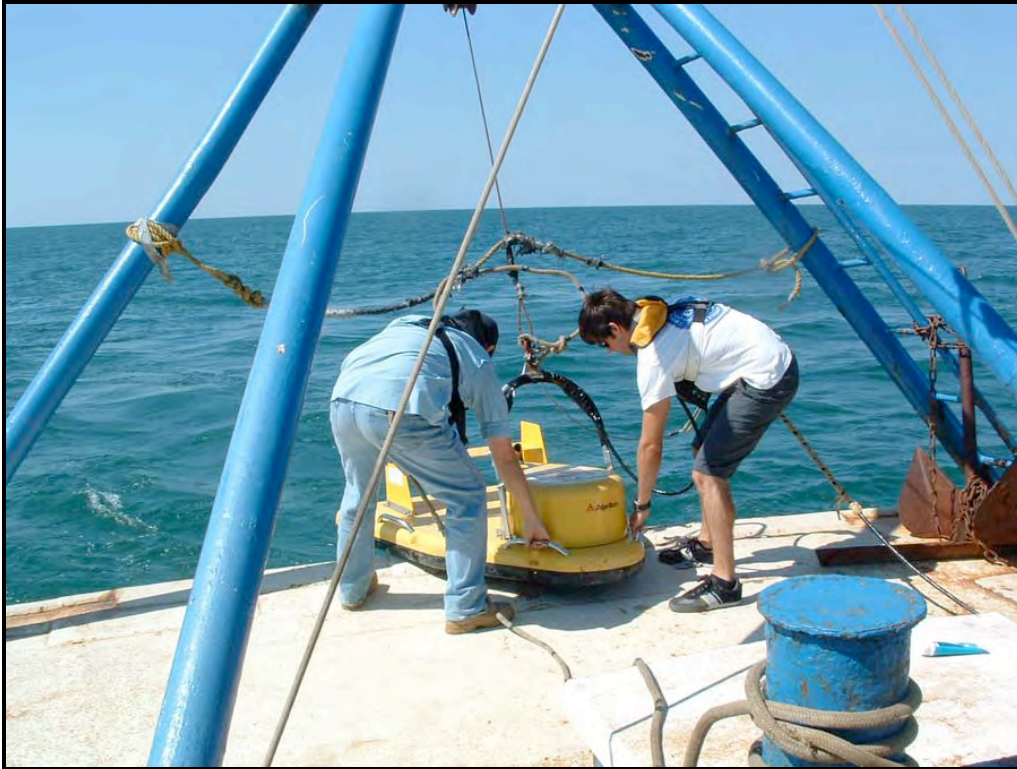
Figure 14. Launching the EdgeTech 512i sub-bottom profiler.
