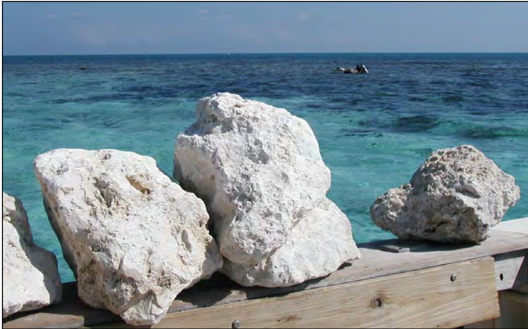
Figure 11 Limestone Boulders (Size Range of 1 to 1.5 feet [0.3 to 0.5 meters]) Representative of Those Suggested for Mitigation to be Used to Mimic the Low-relief Structure of the Natural Hard Bottom Habitat
