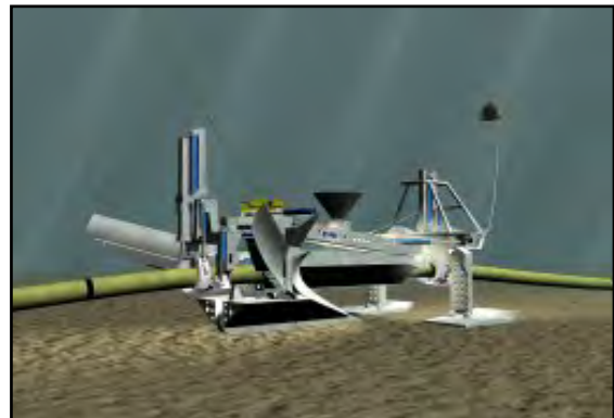
Figure 3-7 Monitoring and Adjustment of Ditch Being Cut
