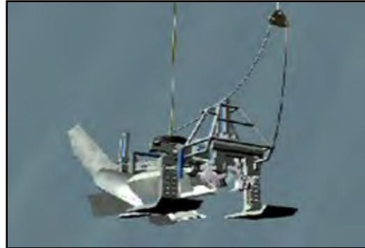
Figure 3-5 Lowering Plow with Share Open
