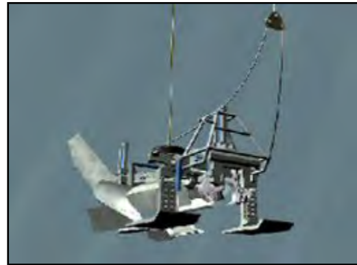
Figure 4-5 Lowering Plow with Share Open
