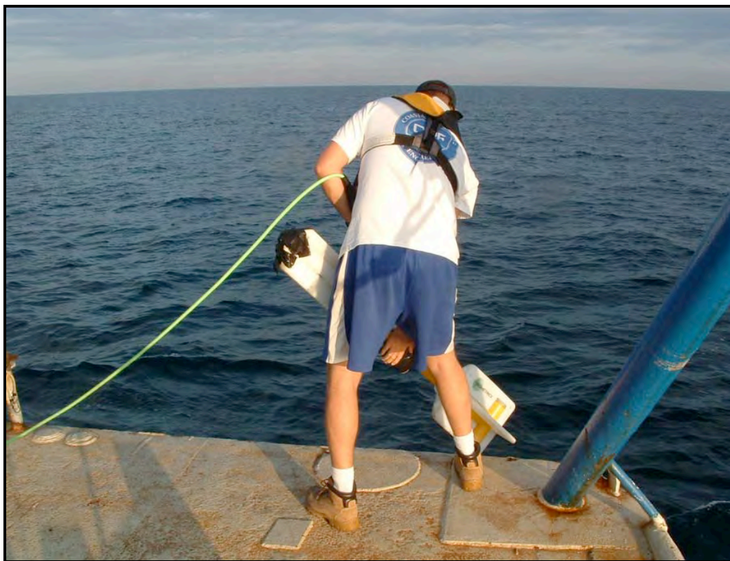
Figure 12. Deploying the EG&G Geometrics G-882 magnetometer.
