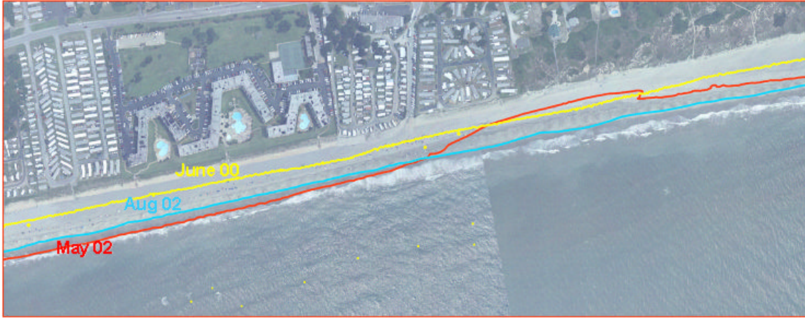
Figure C-11. Shoreline position (MHW) data derived from survey data displaying influence of local beachfill.
