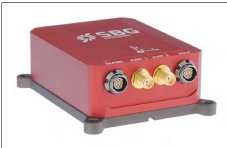
Figure 3-03. SBG Systems Ellipse2-D navigation and inertial compensator used during the investigation.
