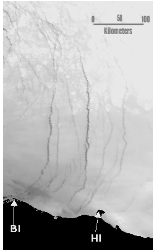
Figure 4.3.22. High angle leads between Barter and Herschel Islands. In this example, the leads tend to curve toward tangency with the edge of the landfast ice, but other characteristics are similar to those in Figure 4.3.21. Symbols are [BI] Barter Island and [HI] Herschel Island. February 14, 2000.
