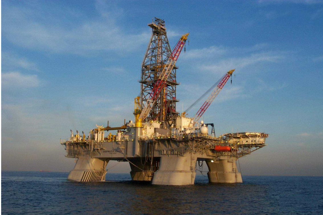
Figure 25. The Deepwater Horizon , a dynamically positioned, semisubmersible drilling unit (photo courtesy of Transocean).
