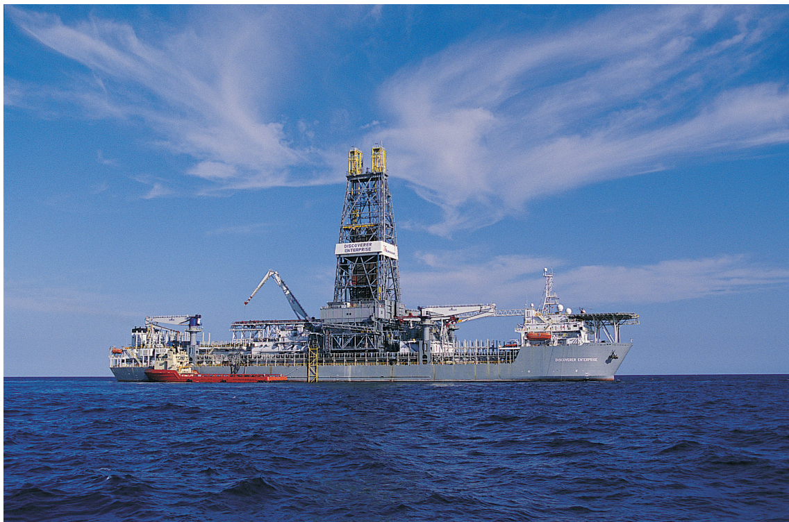
Figure 26. The Discoverer Enterprise , a double-hulled, dynamically positioned drillship (photo courtesy of Transocean).
