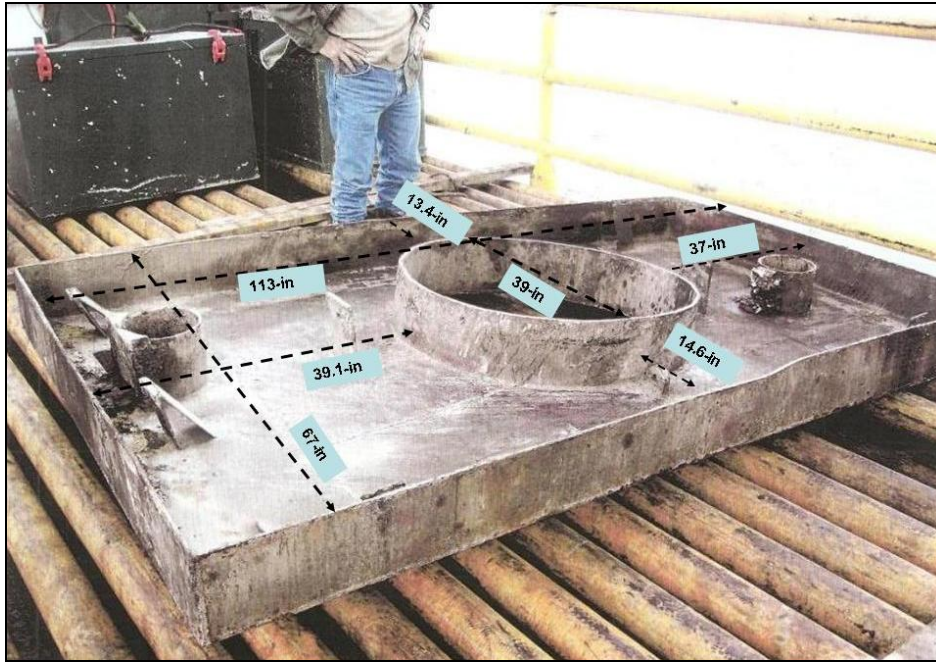
Figure 9 – Dimensions and view of the oil pollution pan
