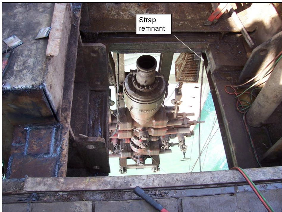
Figure 8 – View down through the rotary table well after fall of the oil pan
