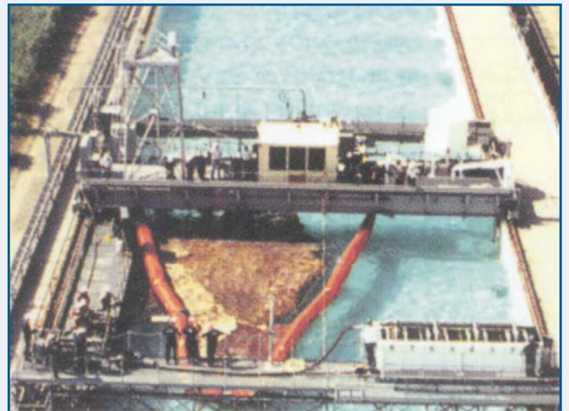
Containment boom and skimmer being tested with oil at the National Oil Spill Response test facility
