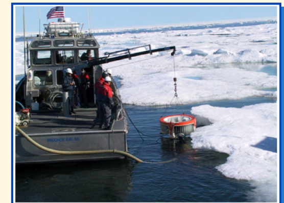
Successful skimming operations demonstrated in broken ice conditions in 2000
