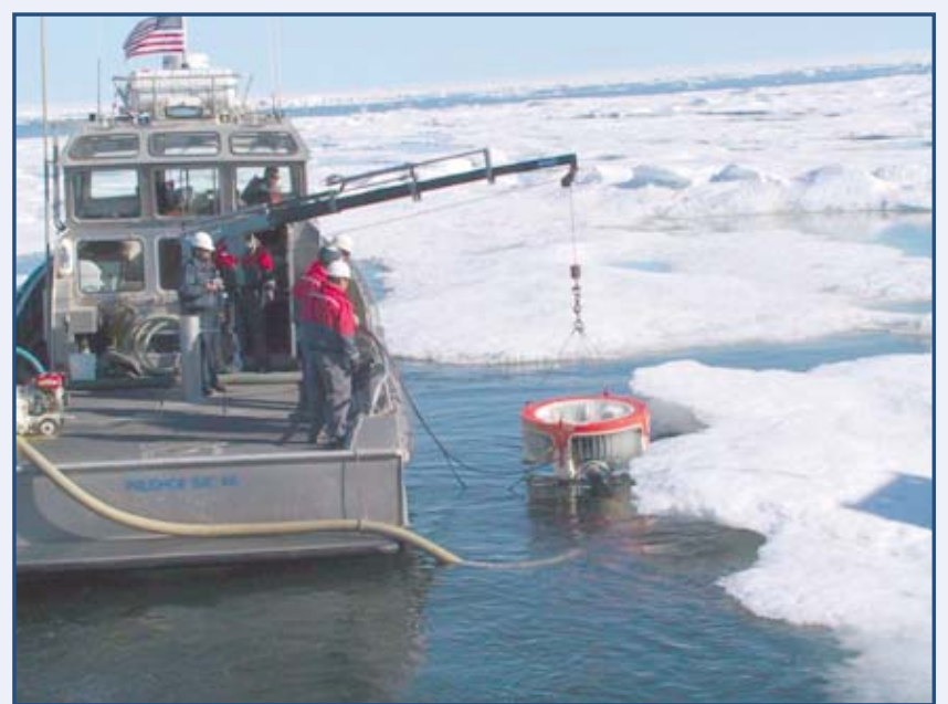
Example of skimming operations in broken ice - 2002
