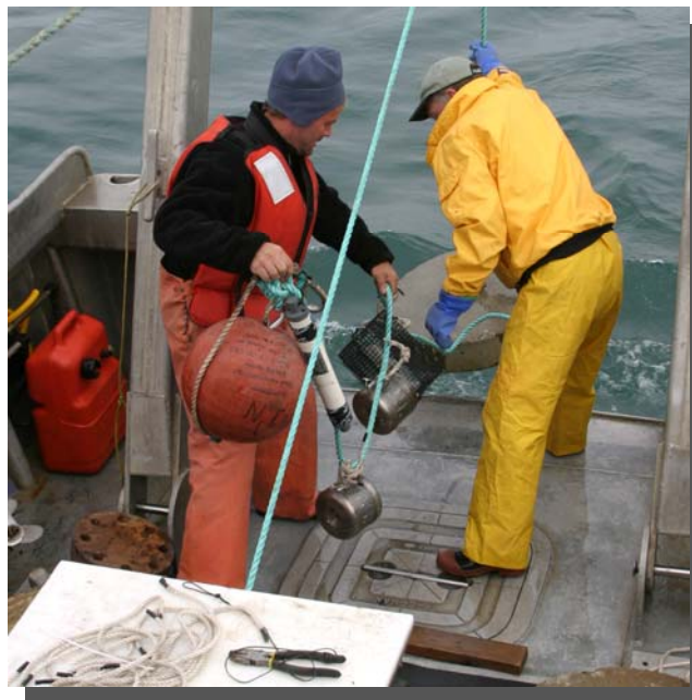
Deploying mussel/SPMD mooring w/acoustic pinger
