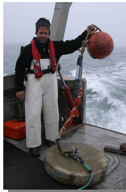
Mussel mooring w/acoustic pinger
