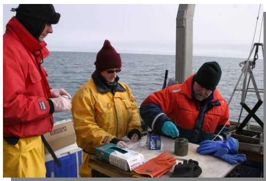
Homogenizing sediment collected from Van Veen grab
