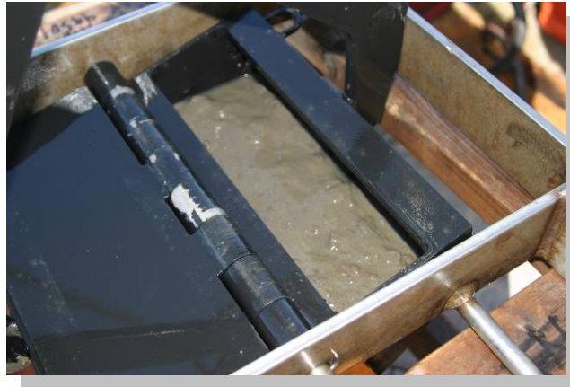
Surficial sediment collected with Van-Veen sampler
