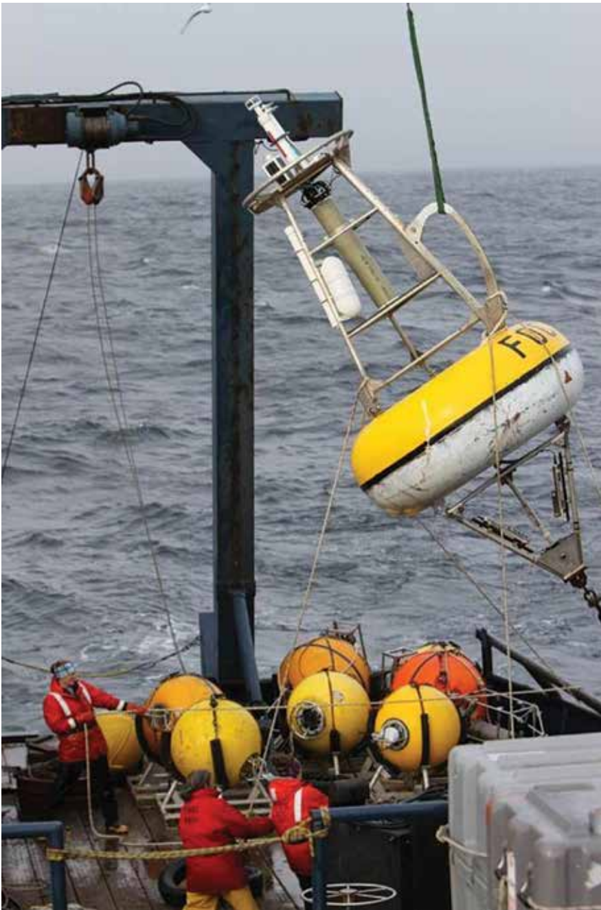
Retrieving a surface-float oceanographic mooring. Photo by Angela Keeling-Garcia.
