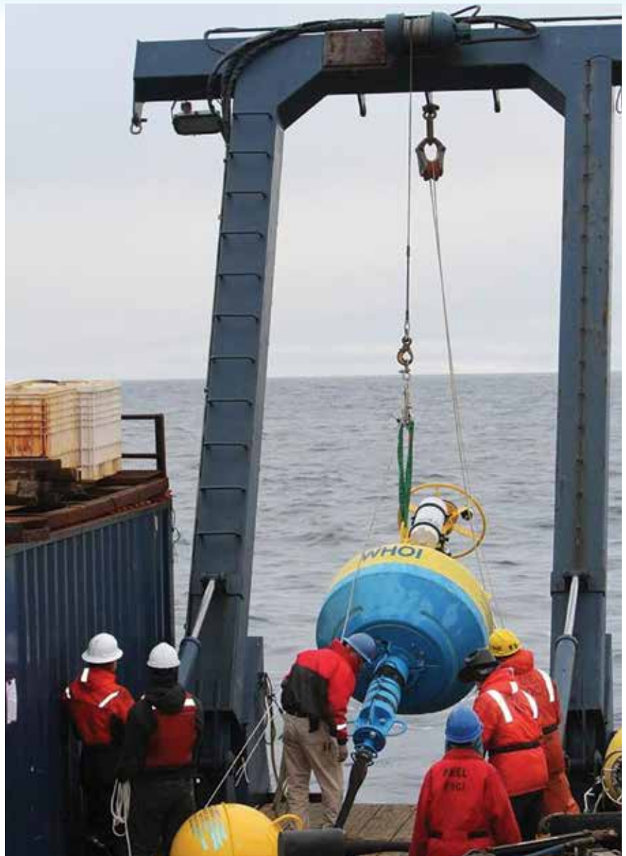
Real-time auto-detection buoy being deployed through the A-frame. Photo by Angela Keeling-Garcia.
