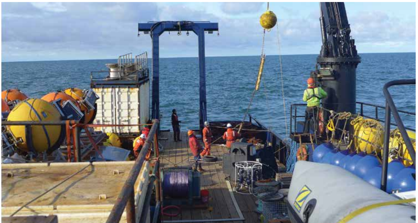
Retrieving a passive acoustic recorder mooring. Photo by Danielle Cholewiak.
