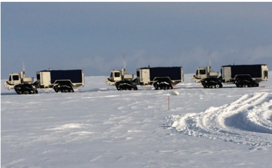
Vibroseis trucks preparing to collect seismic data offshore Alaska.
