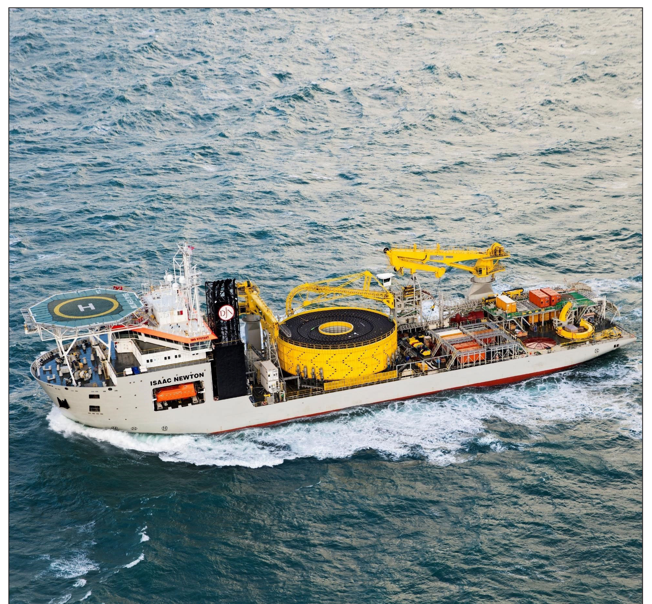
Cable Laying Vessel (Source: Jan De Nul 2020)
