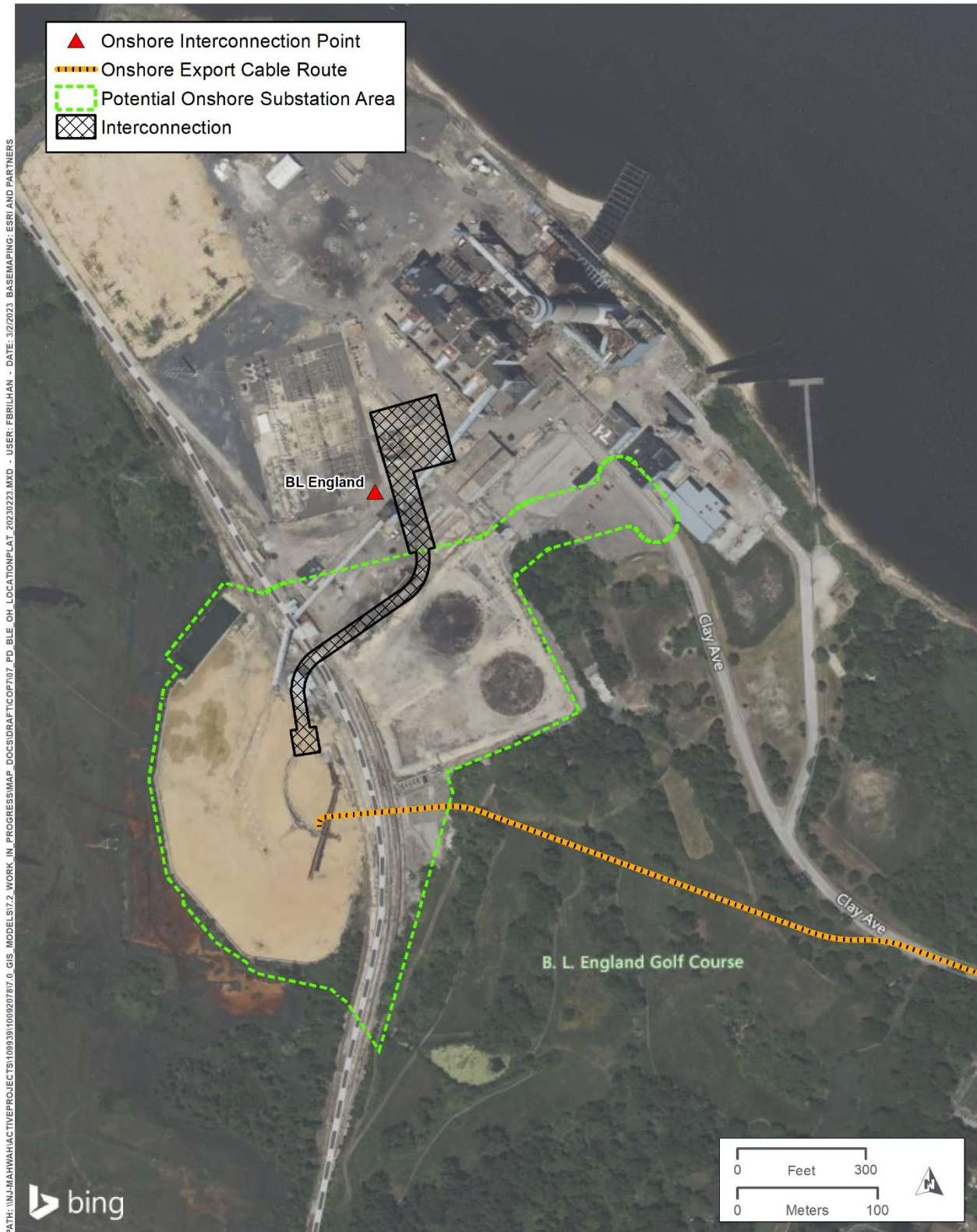
Figure 6.2.1-6. Indicative underground transmission cable route – BL England.
