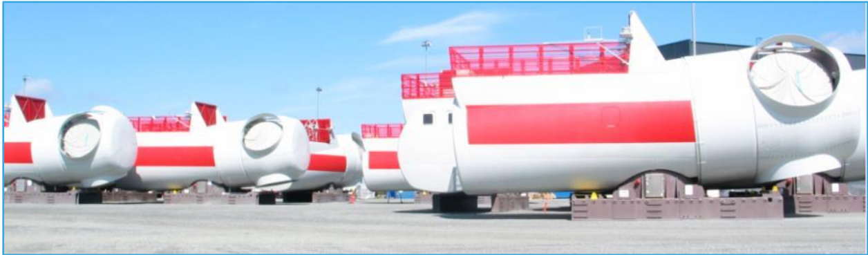
Figure 6.1.2-7. Nacelles pre-assembled and ready at load-out port.
