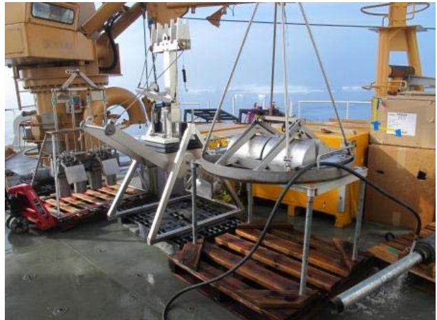
Sampling equipment used to gather sediment and biological specimens during the August 2012 mission. Left to right, multi-Haps core, box core, double Van Veen grab, with missile-shaped gravity cores at each end. Photo: Kathy Kuletz, US Fish and Wildlife Service
