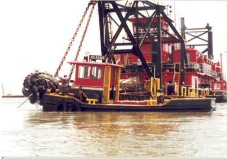
Used a cutterhead dredge to excavate the flotation canal and large slips and pump material where desired
