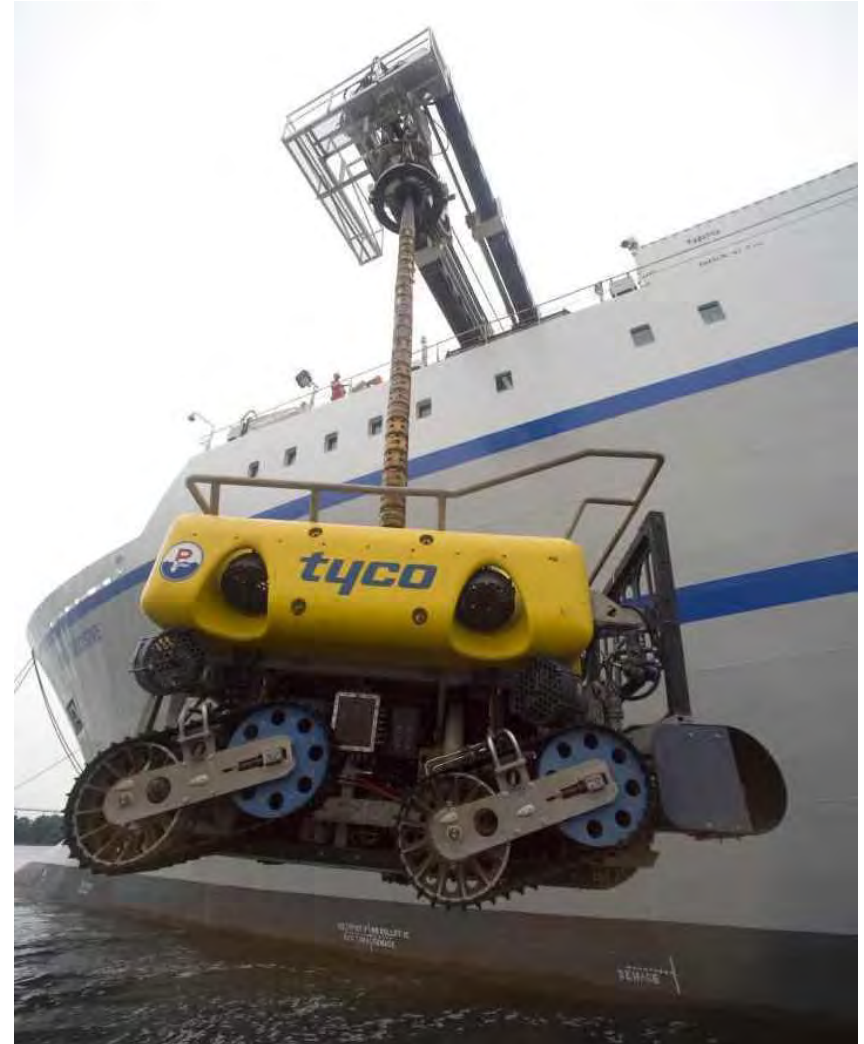
ROV used for cable inspection, recovery and burial Source: TE SubCom
