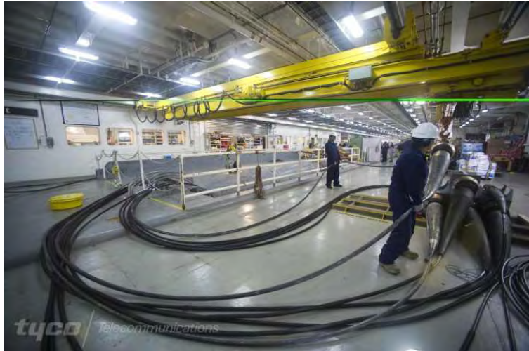
Cable and repeaters inside a cable ship Source: TE SubCom
