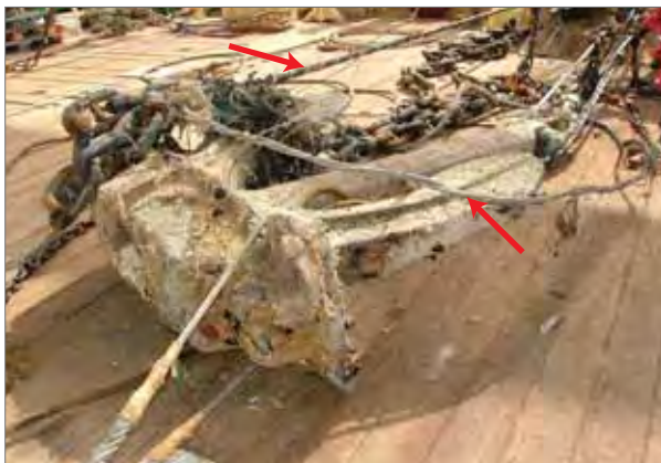
Figure 8.2: As the size and numbers of merchant vessels have increased, so has the risk of damage to submarine cables, as shown by a faulted cable (arrows) entangled with a ship's anchor. Source: unknown.
