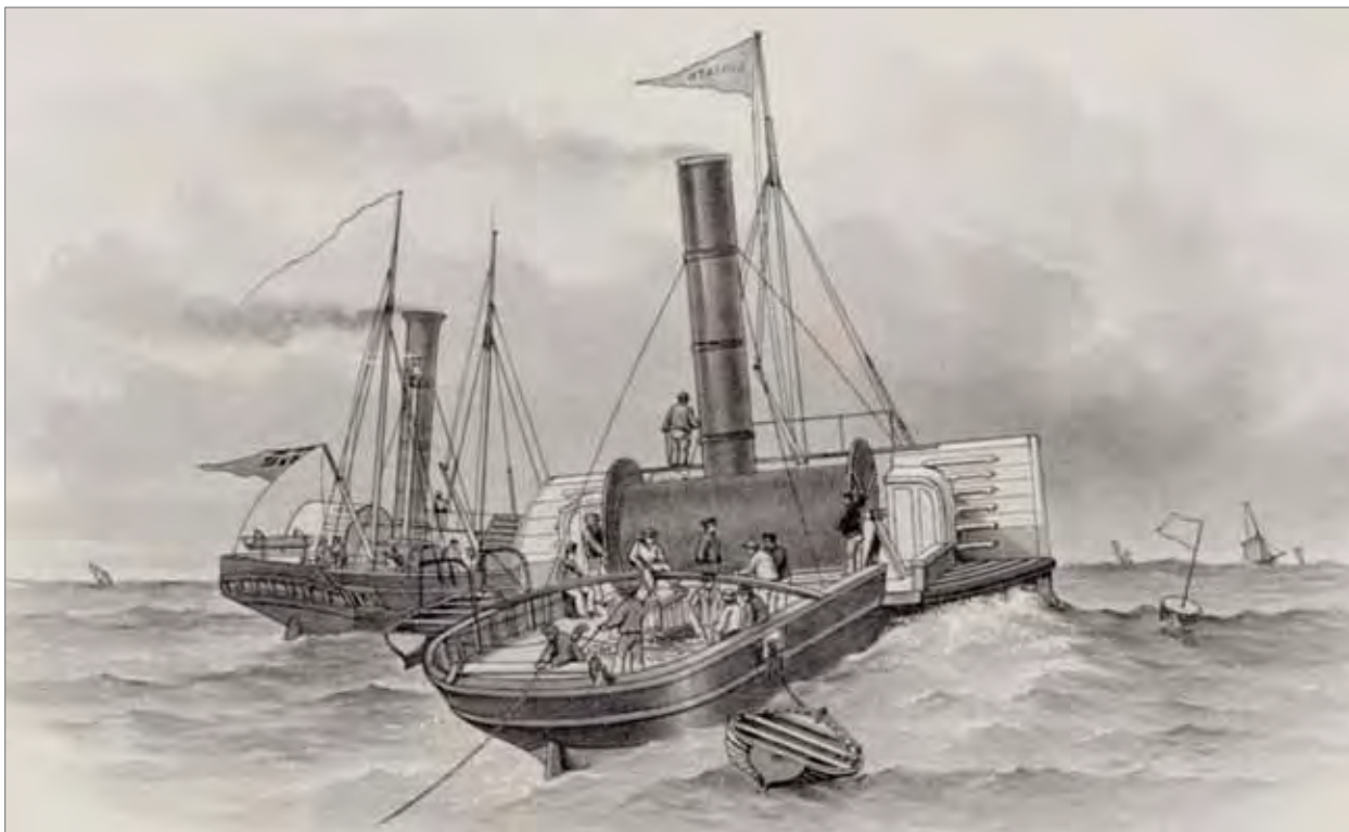
Figure 1.2: The steam tug, Goliath , laying the first international submarine cable between Dover and Calais, 28 August 1850. The vessel was accompanied by HMS Widgeon . Source: Bright (1898).
