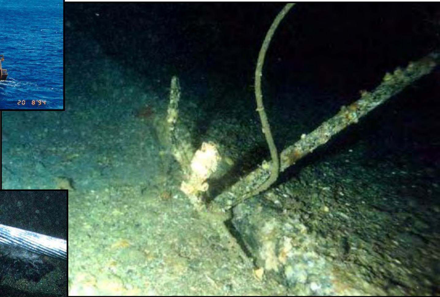
Cable snagged and moved by trawl gear
