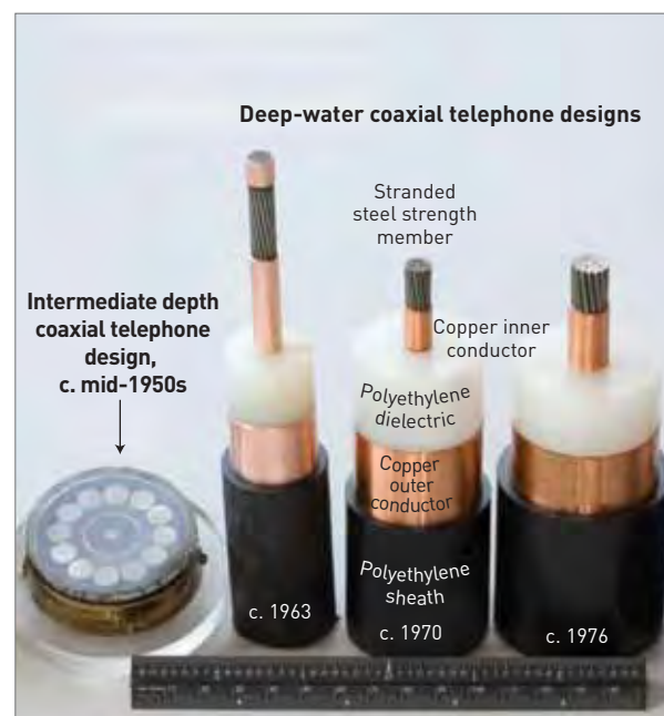
Figure 2.2: Cables of the coaxial telephonic era, with a core of steel wires for strength, an inner copper sheath, which also acted as the conductor, encased in polyethylene dielectric, and an outer conductor. The assembly was coated with black polyethylene which, in shallow water, was armoured for protection. Source: Lonnie Hagadorn.
