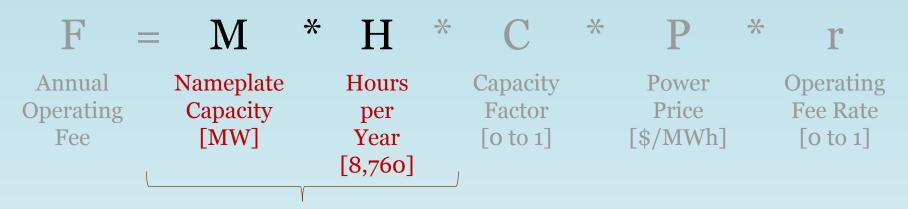
Generation at continuous full power operation (MWh)
