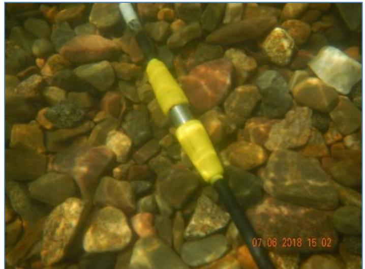
the Dipole-Dipole array with electrode spacing of 3 m along a specially manufactured marine resistivity cable built with 56 stainless steel electrodes. The cable was deployed to rest on the seabed and stabilized with steel weights positioned near the first and last
