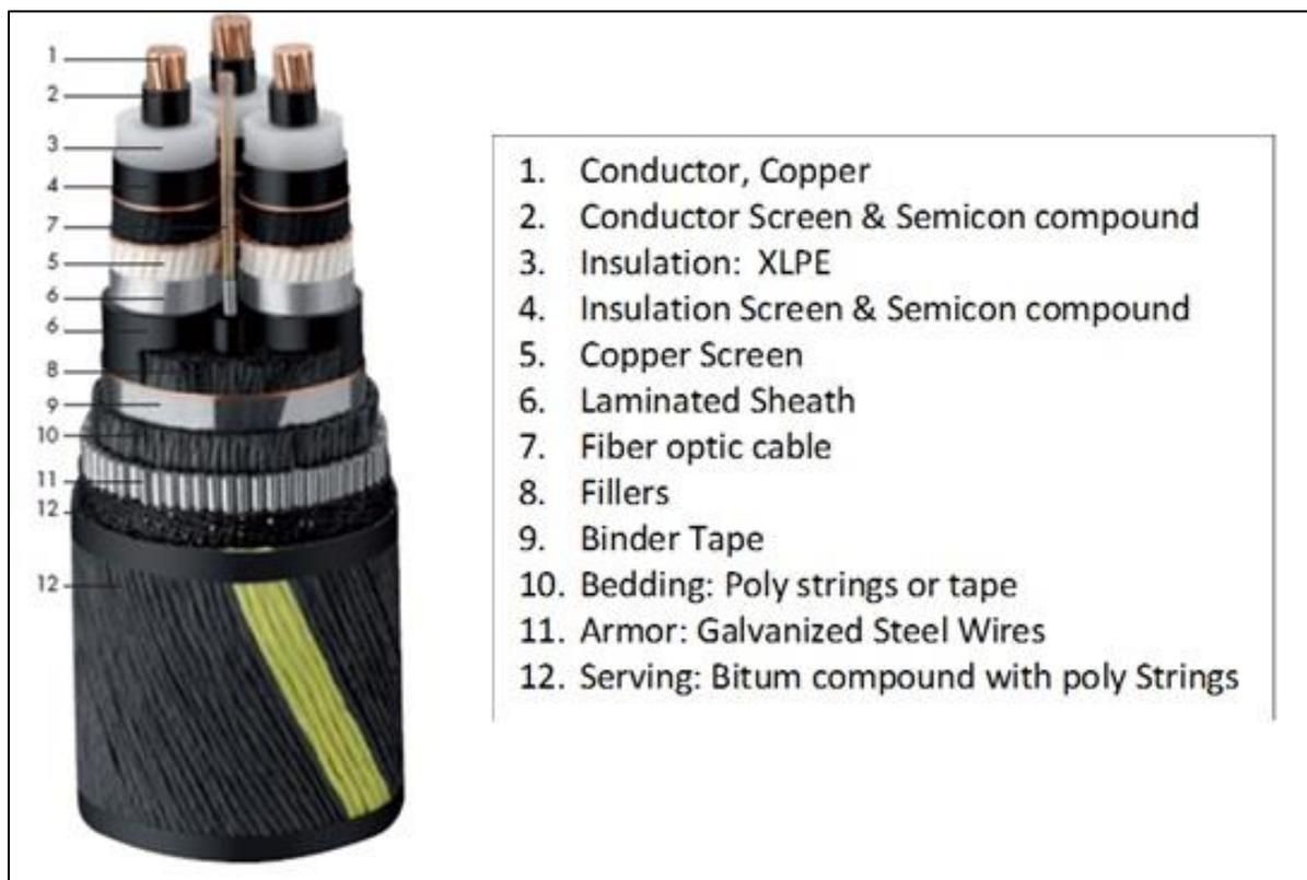
**Figure A-11. Example of medium-voltage subsea cable.**
