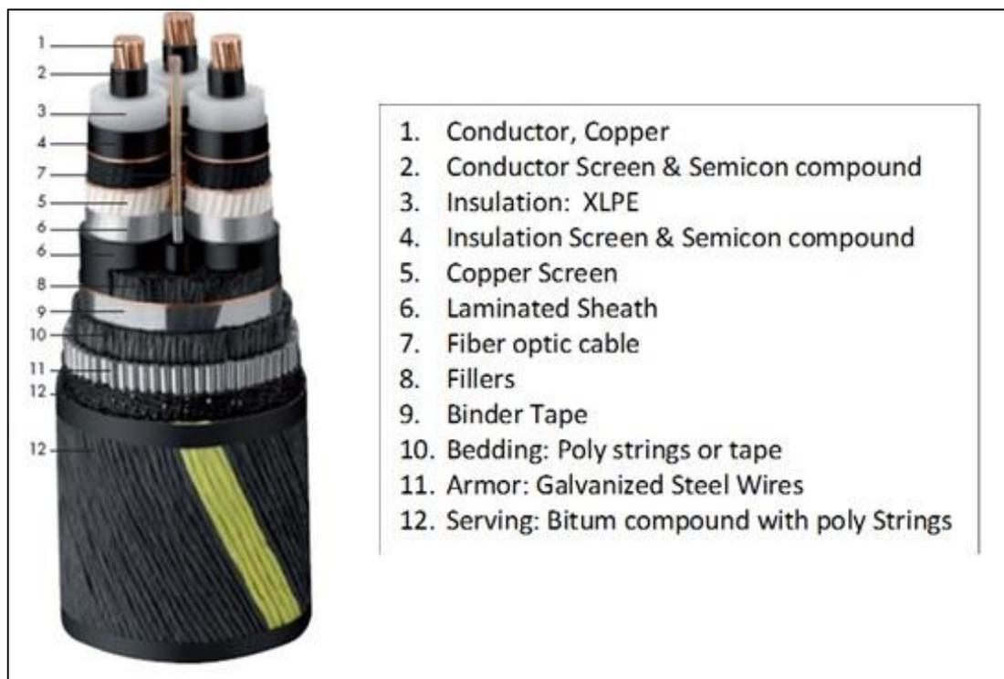
**Figure 2-8. Example of medium-voltage subsea cable.**
