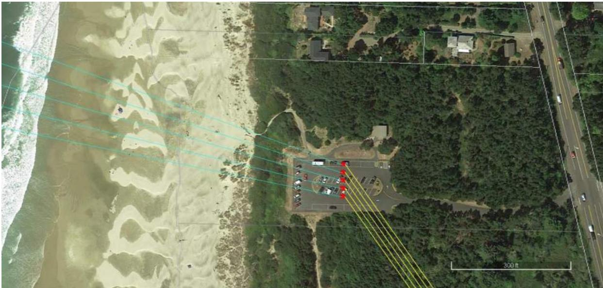
**Figure 3-10. PacWave South landfall, Driftwood Beach State Recreation Site. Beach manholes are shown in red, the buried HDD conduits to the test site are shown in green, and the underground HDD conduits to the Utility Connection and Monitoring Facility are shown in yellow.**
