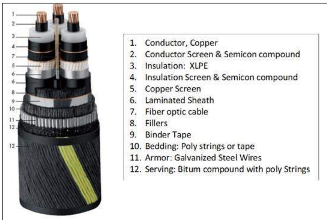
**Figure 2-8.** Example of medium-voltage subsea cable.
