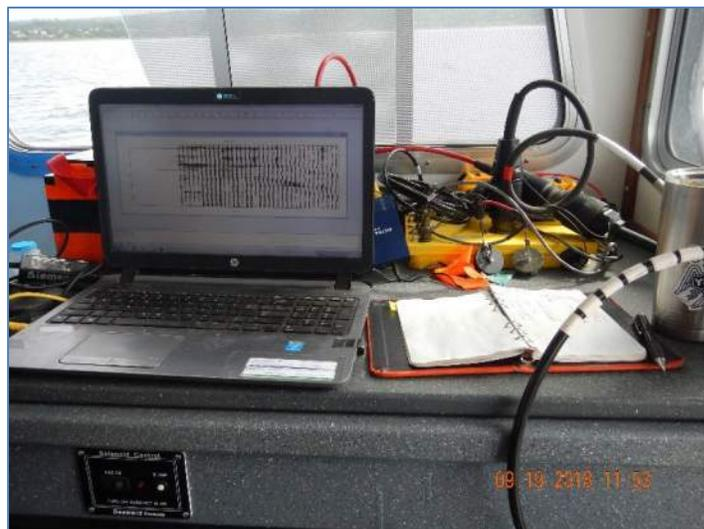
recorded although the records contain significant frequencies related to ocean swell, vessel engine vibrations, and more. Higher frequency input was provided using “Thumper,” a proprietary marine source that was operated from a jet-ski along the hydrophone array.
