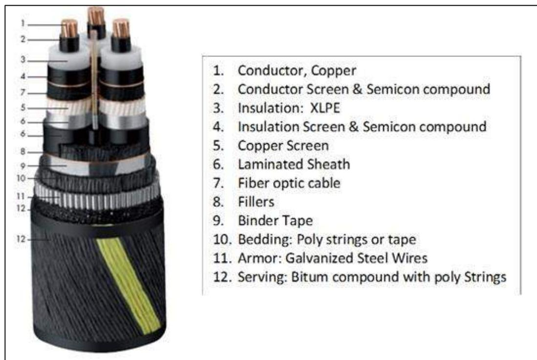
**Figure 3-8. Example of medium-voltage subsea cable.**
