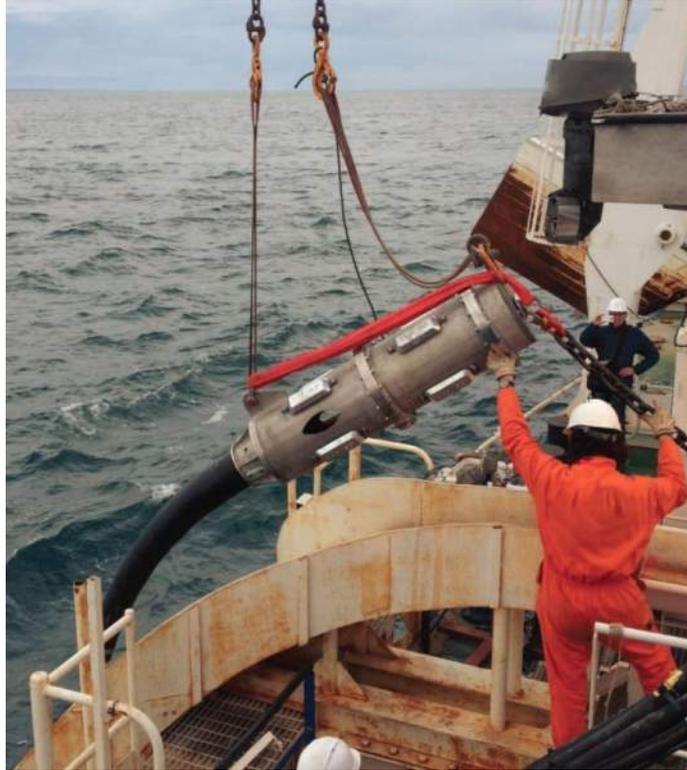
**Figure 3-7. Example of subsea connector (MacArtney’s GreenLink Inline Termination).**
