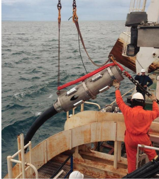
**Figure A-10. Example of subsea connector (MacArtney’s GreenLink Inline Termination).**
