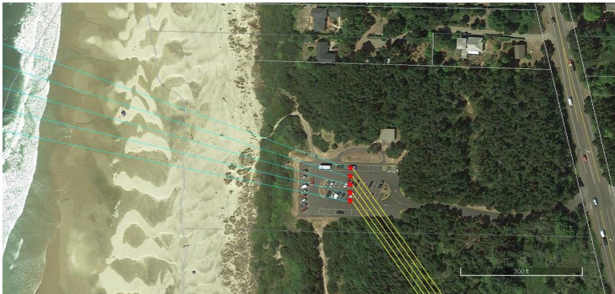
**Figure A-13. PacWave South landfall, Driftwood Beach State Recreation Site. Beach manholes are shown in red, the buried HDD conduits to the test site are shown in green, and the underground HDD conduits to the Utility Connection and Monitoring Facility are shown in yellow.**
