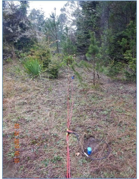
Data were recorded using a networked pair of DAQ 4 seismographs manufactured by Seismic Source in Ponca City, Oklahoma, USA, connected to an IBM laptop computer. Lines were composed of 48 to 96 receivers on 10 foot spacing with shot intervals of 30 feet.
