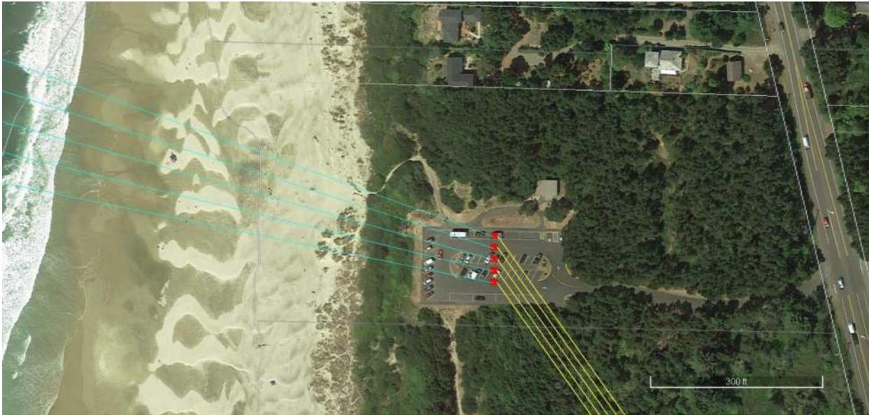
**Figure 2-10. PacWave South landfall, Driftwood Beach State Recreation Site. Beach manholes are shown in red, the buried HDD conduits to the test site are shown in green, and the underground HDD conduits to the Utility Connection and Monitoring Facility are shown in yellow.**
