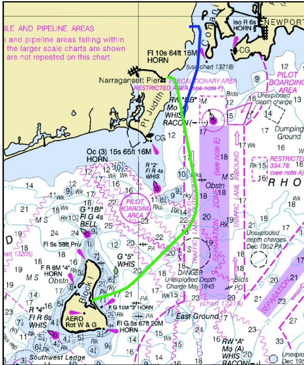
Figure 1. Location map of the areas surveyed in support of the BITS submarine cable route. Green line = primary route, blue line = alternate route. NOAA chart #12300 in background.
