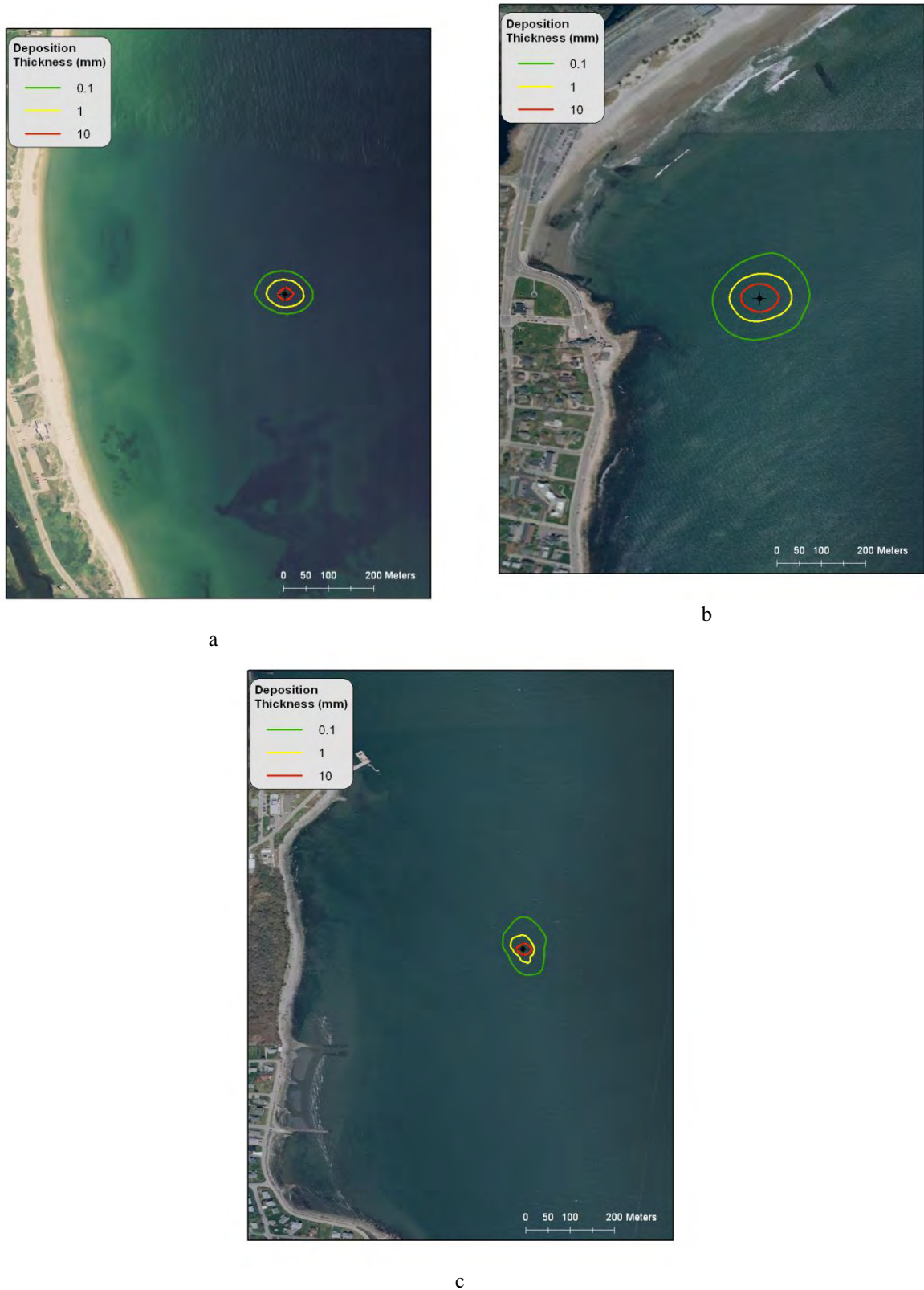
Figure 13. Predicted sediment deposition during refill of the cofferdam off landfalls at a. Block Island; b. Narragansett Town Beach; and c. URI Bay campus. Source: RPS ASA 2012.
