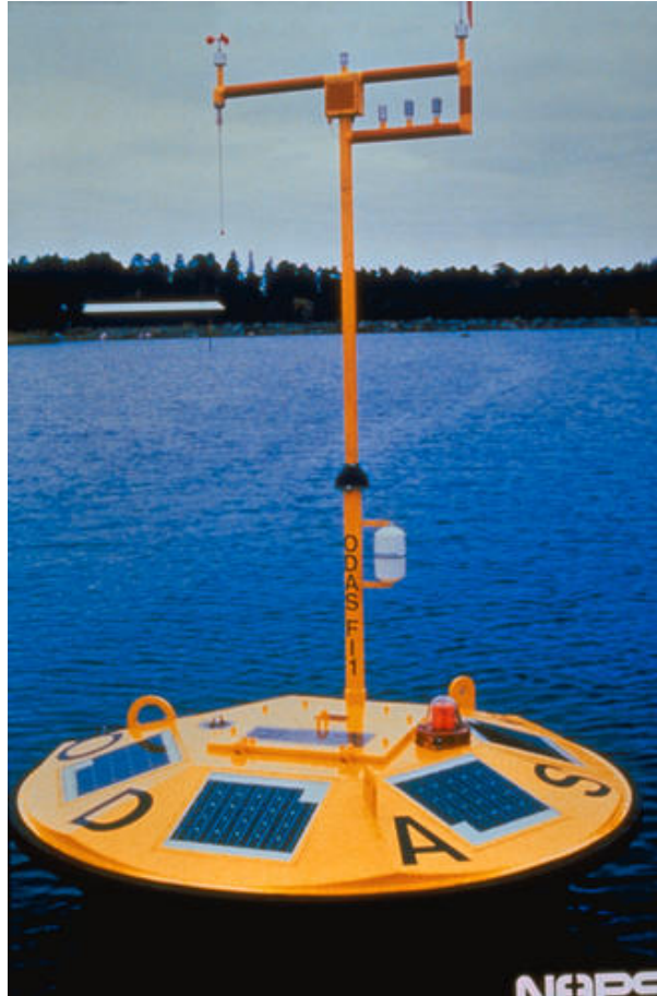
FIGURE 9 Solar-Powered Buoy Used to Collect Weather Data off the Coast of the Eastern United States (Source: NREL 2006b)
