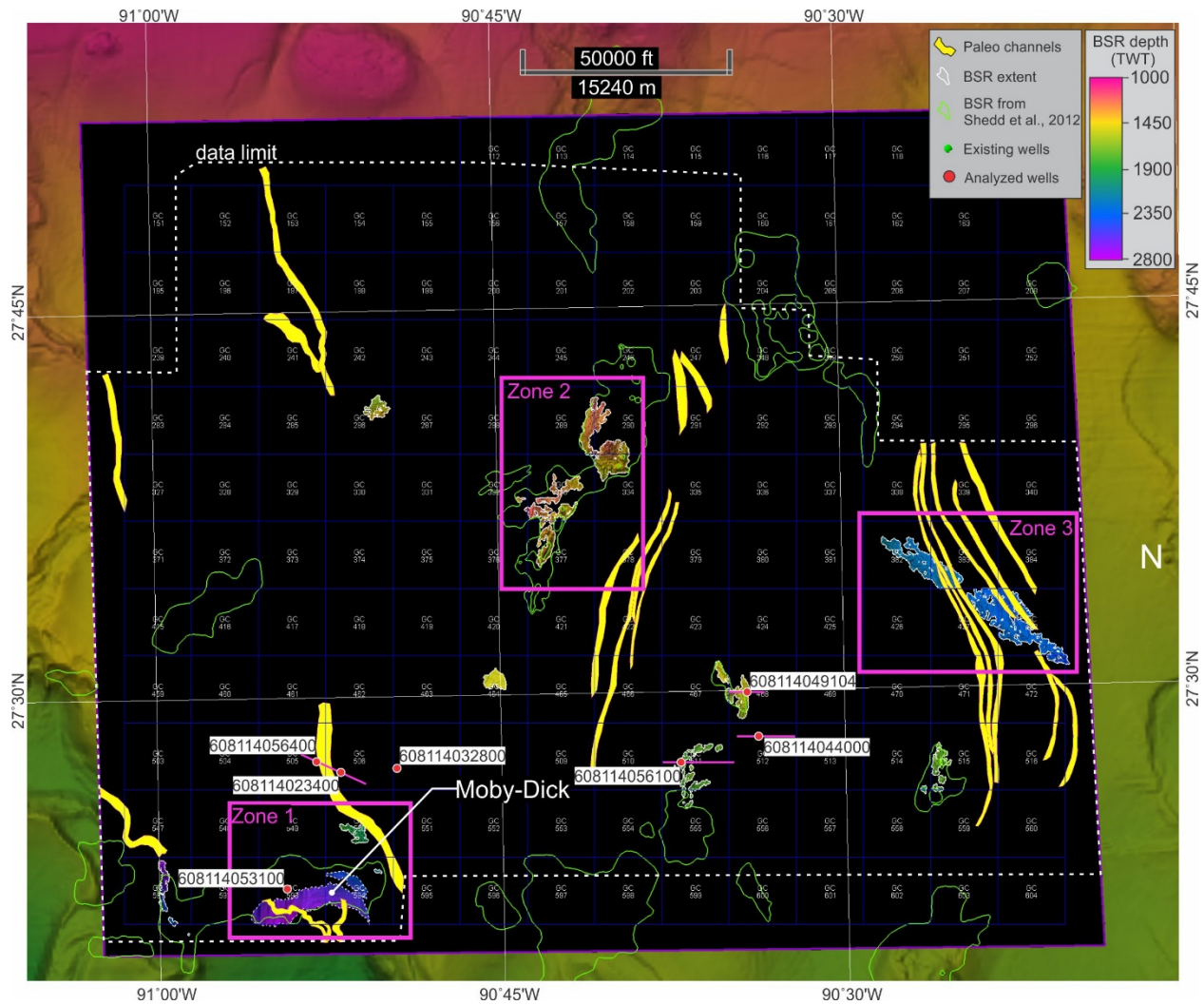
Figure 8. Map showing the depth of the BSRs (msec TWT) identified in the current study. Paleo channels are shown with yellow polygons. Location of a high-confidence Moby-Dick prospect is indicated.
