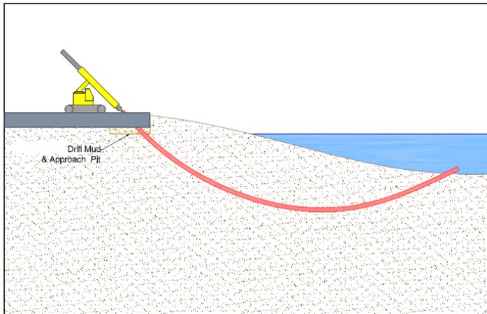
Schematic of typical land-based HDD setup and trajectory
