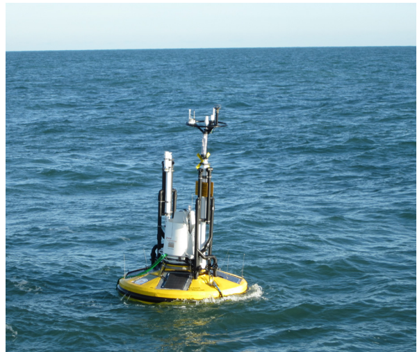
Accurate measurement of wind profile using SEAWATCH Wind LiDAR Buoy
