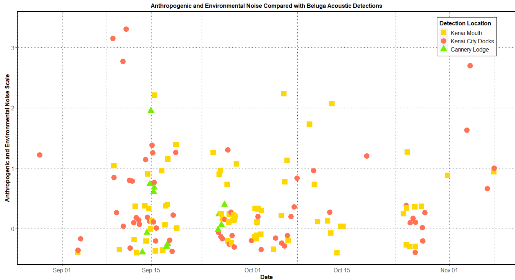
Figure 5. Comparison of beluga acoustic detections in the Kenai River (registered by F-PODs) and anthropogenic and environmental noise (recorded by ST-500). The anthropogenic and environmental noise scale was categorized into 4 different noise categories: 0 representing no noise, 1 representing low noise, 2 representing medium noise, and 3 representing loud noise.
